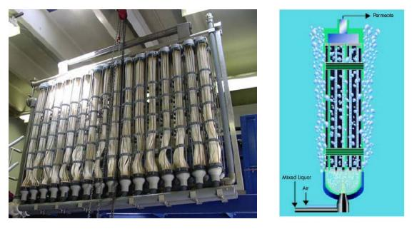
Figure 11: USFilter Hollow Fiber Membrane Module Rack and Memjet System (www.usfilter.com)
