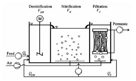
Figure 5: Pilot Municipal Treatment MBR Process Schematic (Rosenberger et al, 2002)
