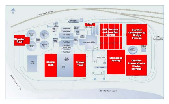
Figure 6: Traverse City MBR Design Layout (Crawford and Lewis, 2005)
