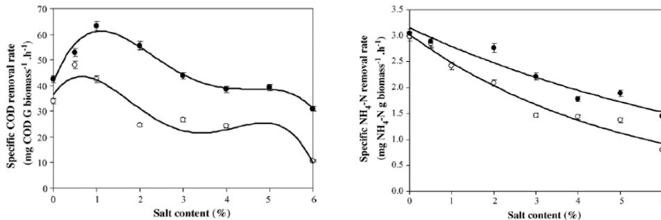
Fig. 3 Variation of specific COD,  $\text{NH}_4 - \text{N}$  and  $\text{PO}_4 - \text{P}$  removal rate with salt content. (Ahmet, 2006)
