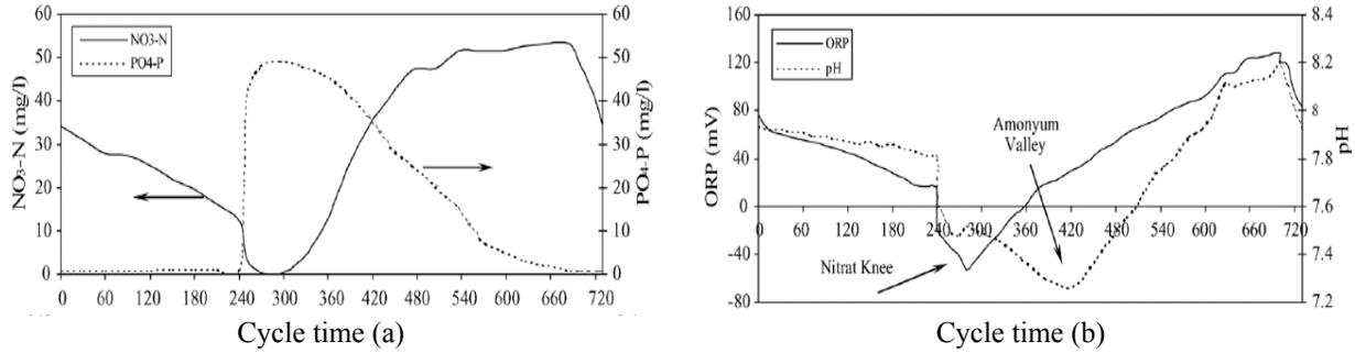
Fig. 4. (a) Nitrate and phosphate, (b) ORP and pH profiles. . (Akin et al., 2005)
