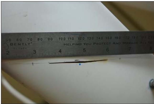
Figure 6 Surface Crack
