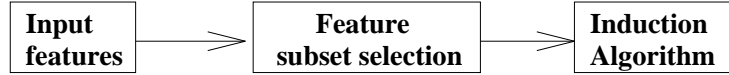
Figure 1.2 The feature filter approach, in which the features are filtered independently of the induction algorithm.
