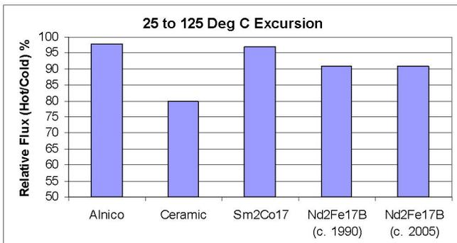
Fig. 1(c) Temperature Impact on Reversible Flux Loss
