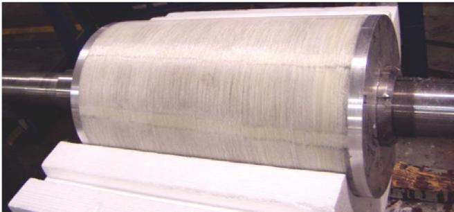
Fig. 12 – Surface PM Rotor
