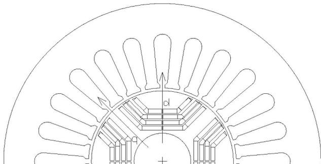
Fig. 5 Interior PM Motor with Multiple Flux Barrier Rotor Saliency
