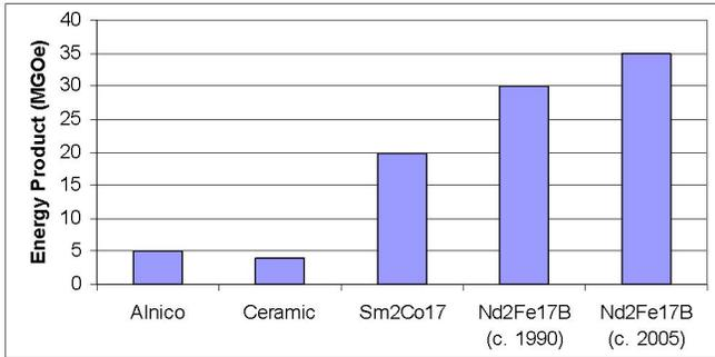
Fig. 1(a) Maximum Energy Product of Various Permanent Magnet Materials
