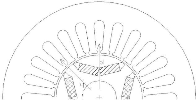
Fig. 4 Interior PM Motor with Rotor Saliency via a Single Flux Barrier
