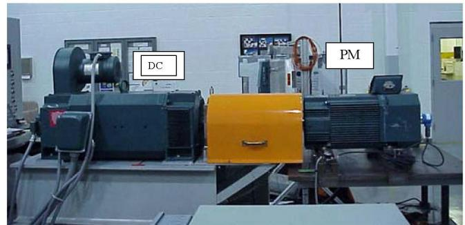
Fig. 11 – 75 HP, TEFC PM Motor (on right) – Coupled to DC Load Motor
