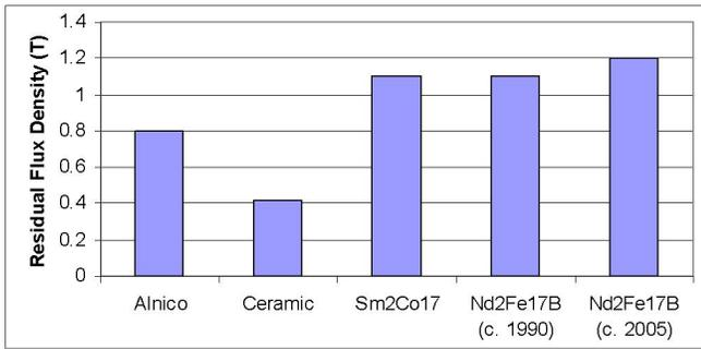
Fig. 1(b) Magnet Residual Flux Density
