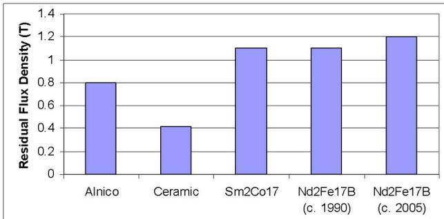
Fig. 1(b) Magnet Residual Flux Density
