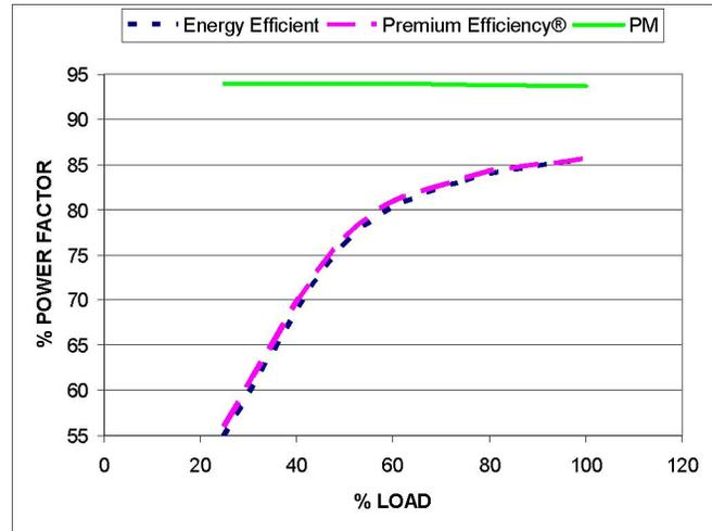
Fig. 10(b) – Typical Partial Load Power Factors of 75 HP, TEFC, 1800 RPM Induction and PM Motors
