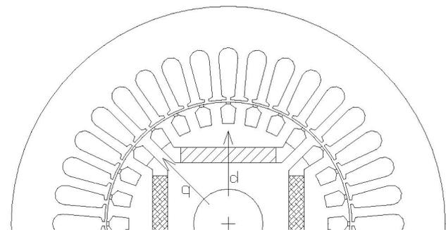
Fig. 6 Interior PM Motor with Rotor Saliency via a Single Flux Barrier – and a Squirrel Cage Winding for Line Starting
