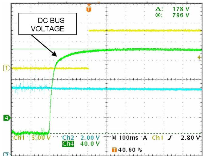
Fig. 8 – DC Bus Voltage Increase Due To Inverter Trip While at 7200 RPM on a 5000 RPM Base Speed PM Motor
