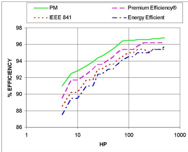
Fig. 9 – Efficiencies of Low Voltage, TEFC, 1800 RPM Induction and PM Motors
