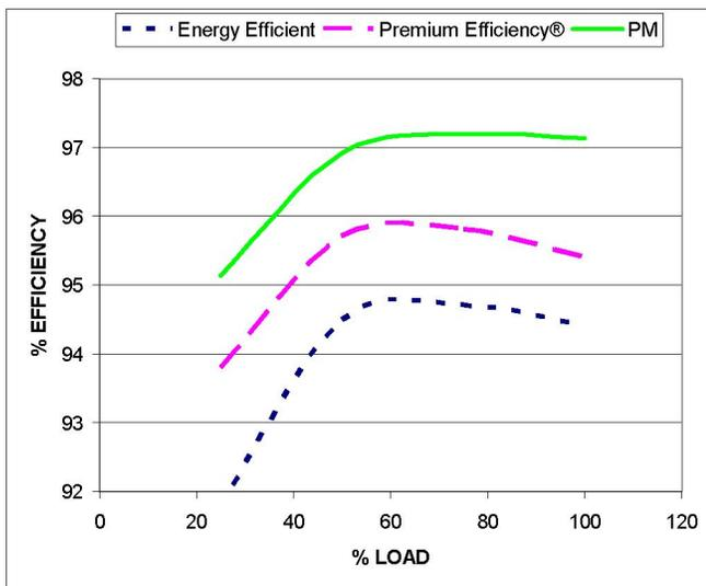
Fig. 10(a) – Typical Partial Load Efficiencies of 75 HP, TEFC, 1800 RPM Induction and PM Motors
