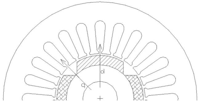
Fig. 2 Surface PM Motor with No Rotor Saliency
