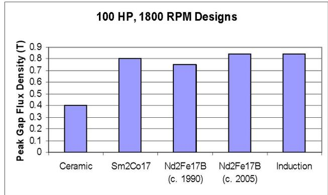
Fig. 1(e) Peak Motor Air Gap Flux Density
