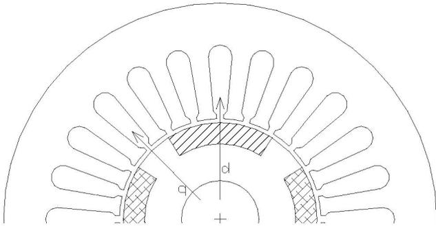
Fig. 3 Surface PM Motor with Teeth Between Magnets to Create Rotor Saliency
