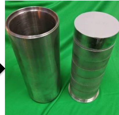
Extrusion can loaded with compacts
