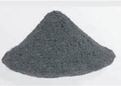
High purity atomized Al (88.5 vol. %)
