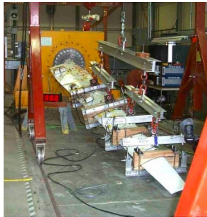
Figure: Instrumented blade ready for loading (Sundaresan, 2002)
