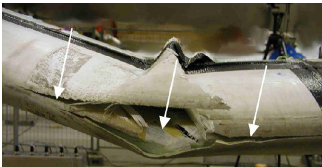
Figure 9. Damage type 2 (adhesive joint failure between skins) at the leading edge [18].
