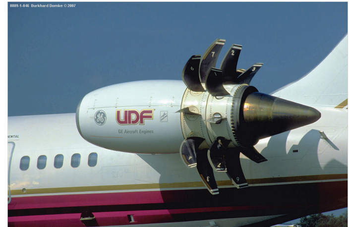
Fuselage-mounted, pusher configuration
