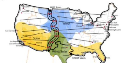
Design 2A: Reconfigured seam - additional B2B capacity only
