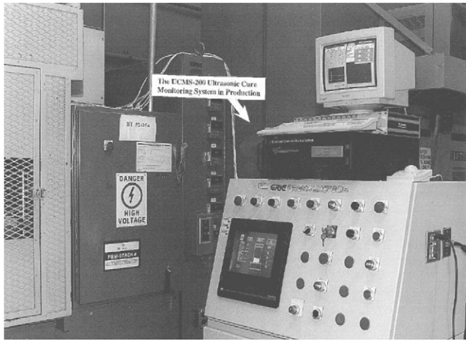
Fig. 19. Automated ultrasonic cure monitoring in an industrial application [21].
