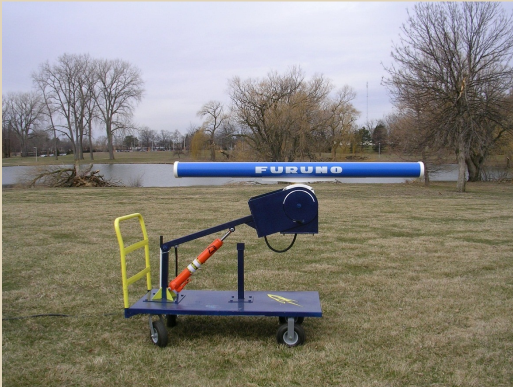
Marine Radar -- Furuno 1525 MK3 - 25 kW radar unit (range scales 1/8-96 n.mi.) with a 6.5 ft. horizontal array antenna and a digitizing card XIR3000 by Russell Technologies Inc
