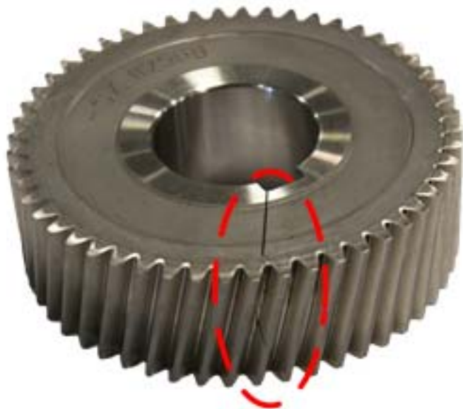
Test gear with a crack
