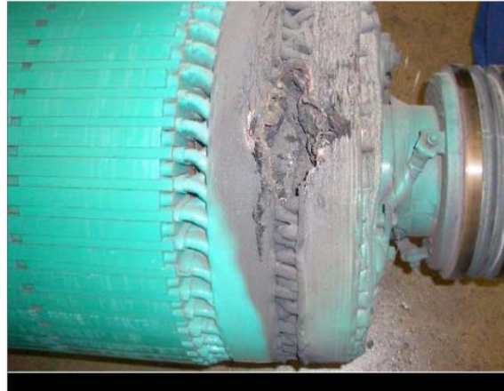
DFIG: insulation failure
