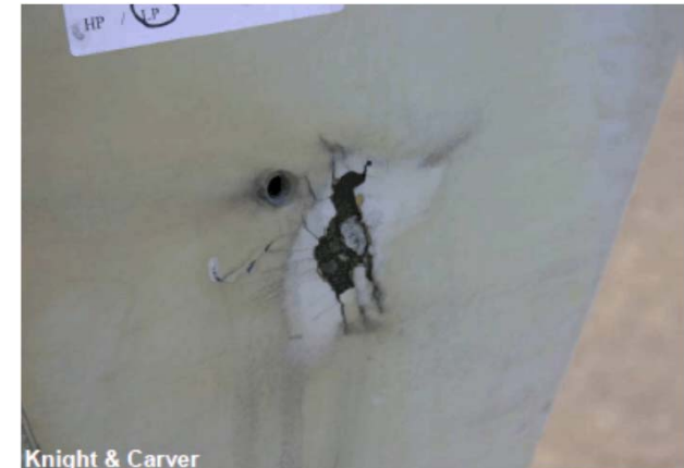
Blade damage: lightning strike
