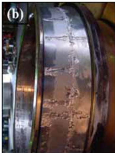
Main shaft bearing: wear tracks on raceway
