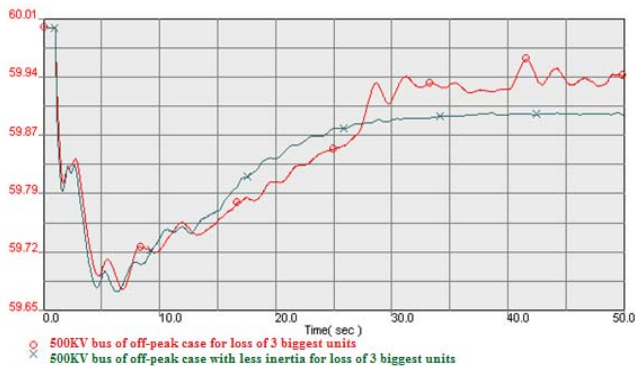
Fig. 5. Circle is off- Peak Case, Star is off-peak case with lower inertia
