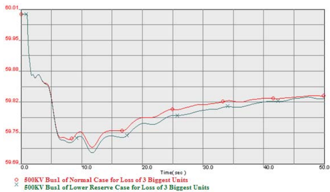
Fig. 6. Circle is peak case; Star is peak case with less governor control
