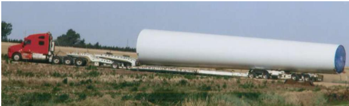
Figure 2.1: Transportation of a Steel Tower (Courtesy of T. Baird, Iowa State University)
