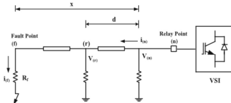
Figure 15. Fault distance calculation using two voltage dividers
