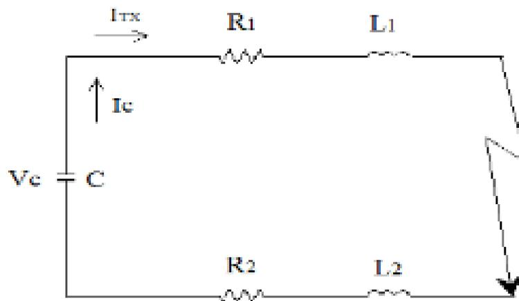
Figure 7. Equivalent circuit of capacitor discharge stage
