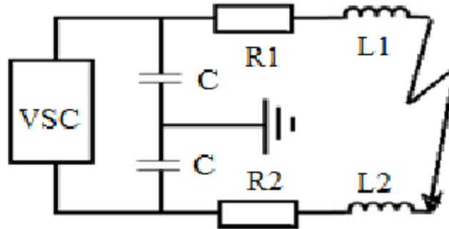
Figure 6. DC LTL fault equivalent circuit
