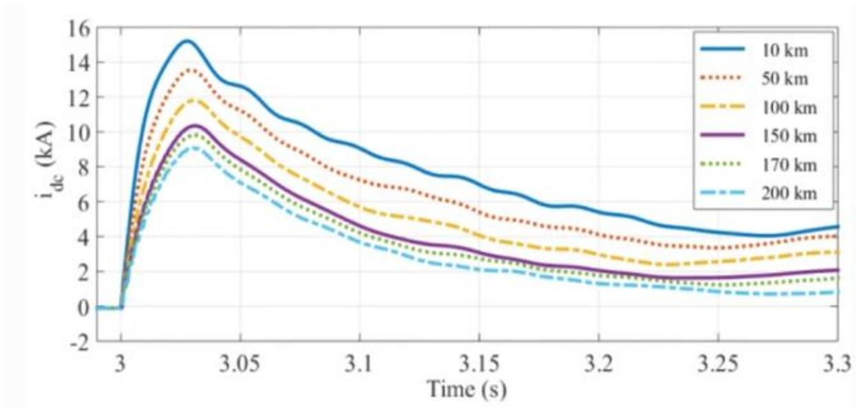
Figure 5. DC LTG fault current ( $i_{dc}$ )
