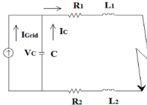
Figure 11. Equivalent circuit of grid current feeding stage stage
