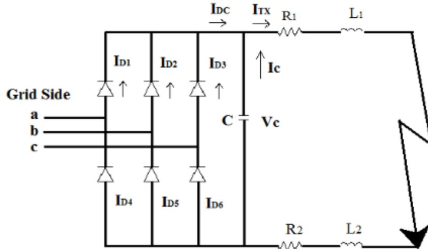
Figure 10. Equivalent circuit of diode freewheel stage
