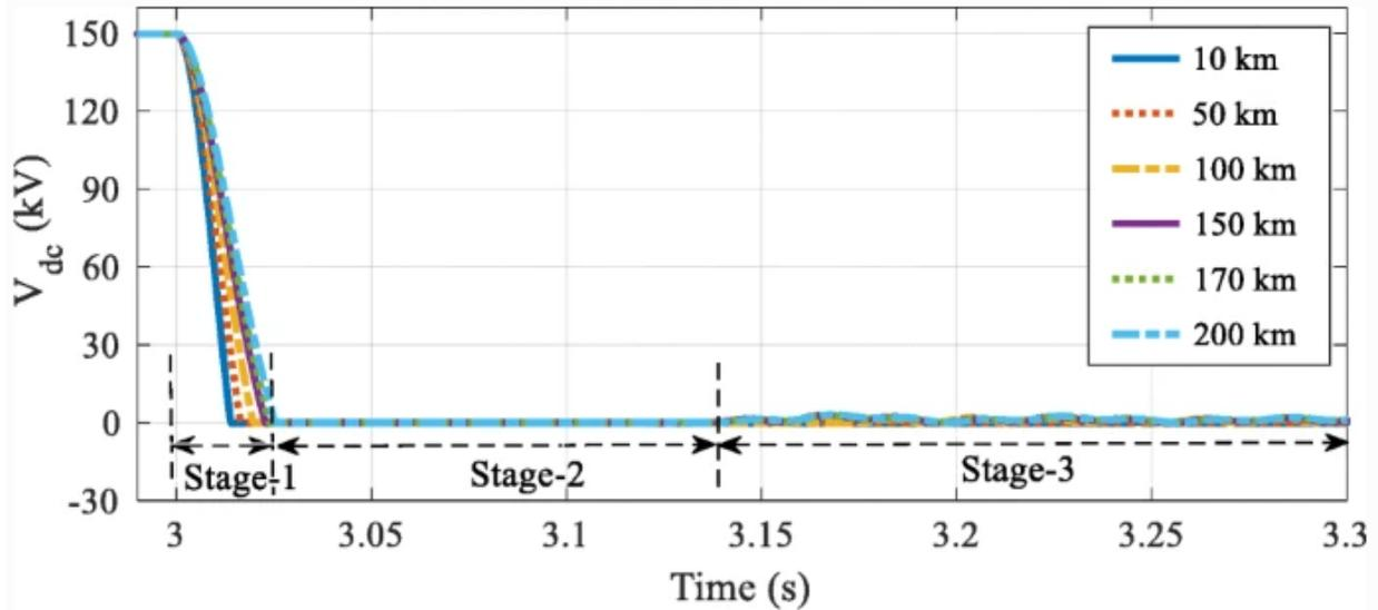
Figure 12. DC DLTG fault positive voltage ( $V_{dc}$ )
