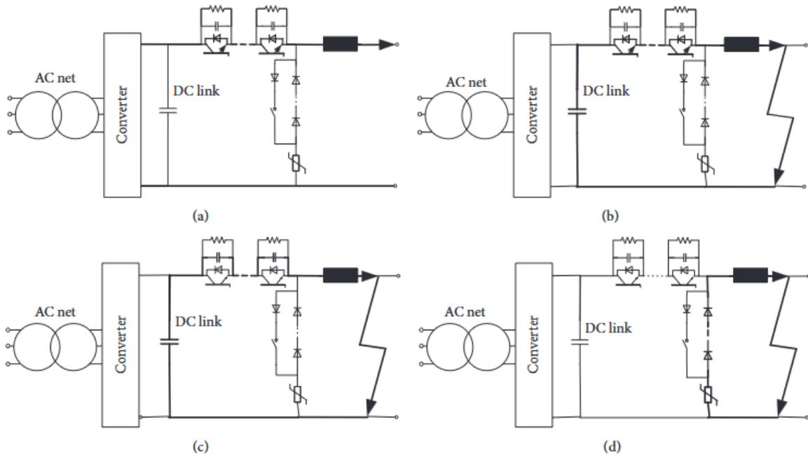
Figure 19. Structure and working principle of all-solid DCCB (a) Normal operation of all-solid HVDC. (b) Short circuit fault occurs. (c) The paralleled capacitor of each IGBT is charged through the loop. (d) The rest energy is consumed in the designed loop.
