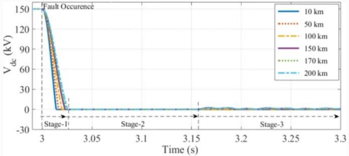
Figure 8. DC LTL fault positive voltage ( $V_{dc}$ )
