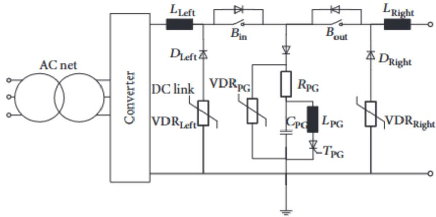
Figure 20. Structure of resonant DCCB
