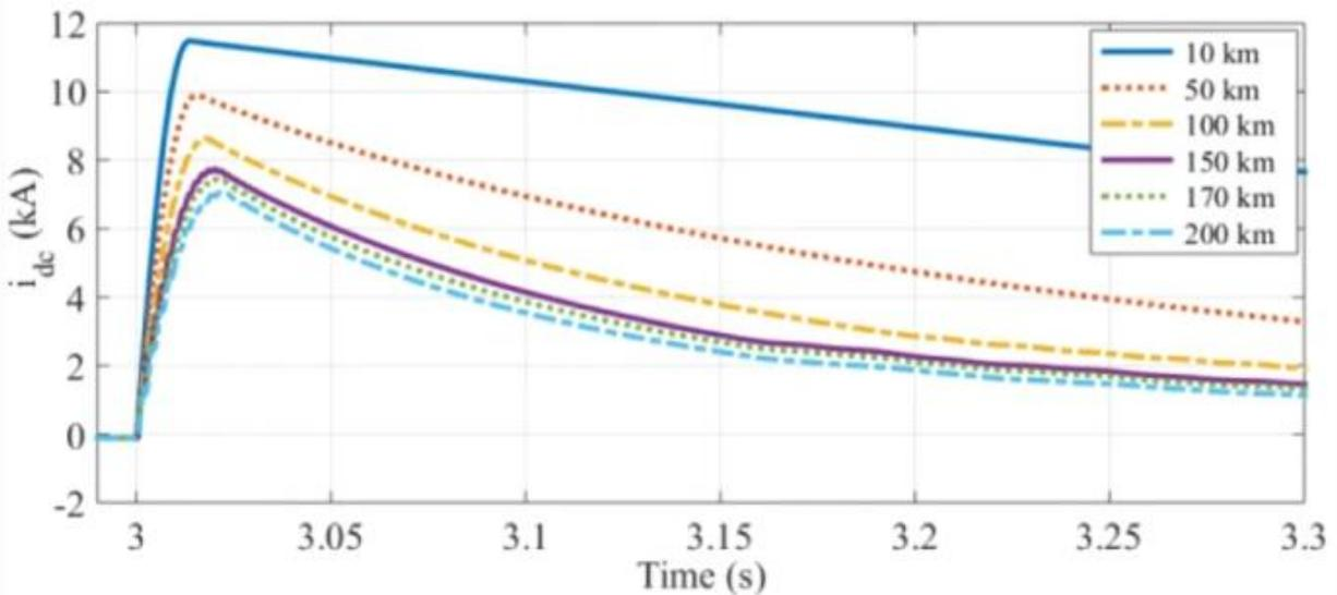
Figure 9. DC LTL fault current ( $i_{dc}$ )
