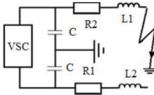
Figure 1. DC LTG fault equivalent circuit
