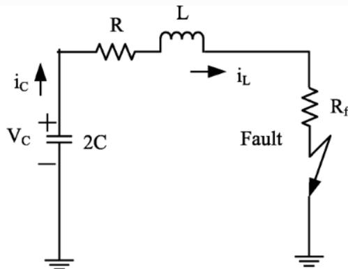
Figure 2. DC LTG fault capacitor discharge equivalent circuit
