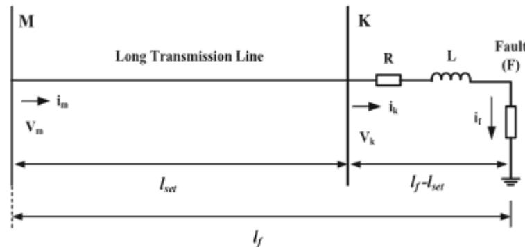
Figure 16. Transmission line model under fault (F) condition
