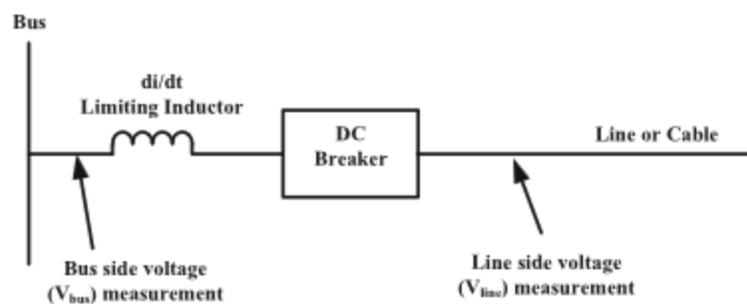
Figure 18. Illustration of fault detection method
