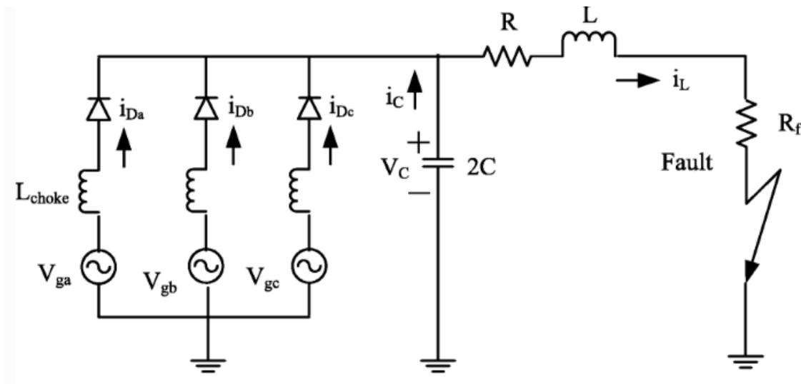
Figure 3. DC LTG fault grid current feeding equivalent circuit
