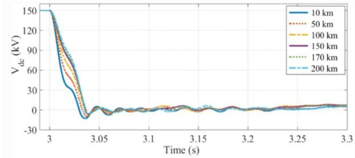
Figure 4. DC LTG fault positive voltage ( $V_{dc}$ )
