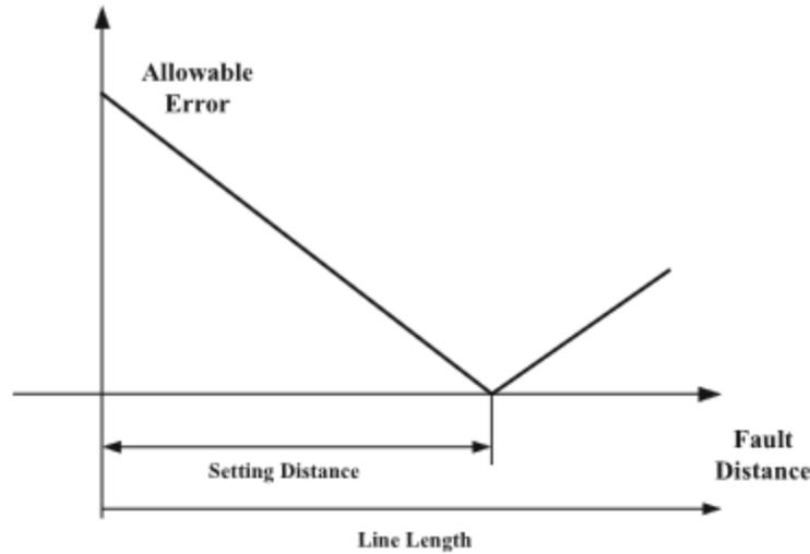
Figure 17. Allowable error vs fault distance
