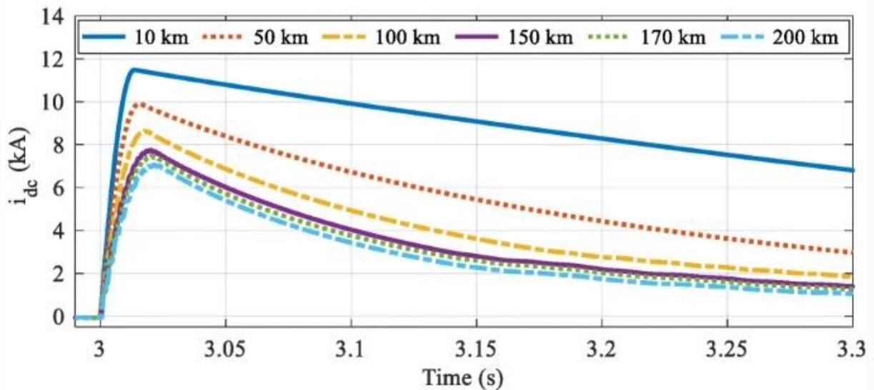
Figure 13. DC DPTG fault current ( $i_{dc}$ )
