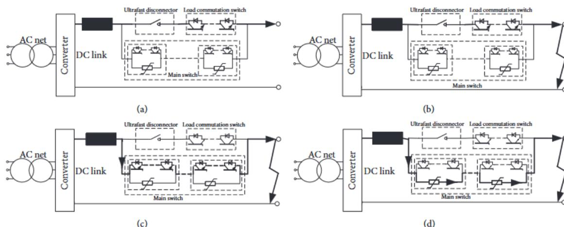
Figure 21. Structure and working principle of hybrid HVDC breaker. (a) Normal operation of hybrid HVDC breaker. (b) Short circuit faults occur and LCS is blocked. (c) Fault current commutates to main switch and UFD is turned off. (d) IGBTs in main breaker are blocked and fault current commutates to arrestors' branch
