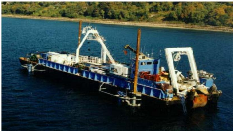
Barge (Shallow Water Cable Installer)
