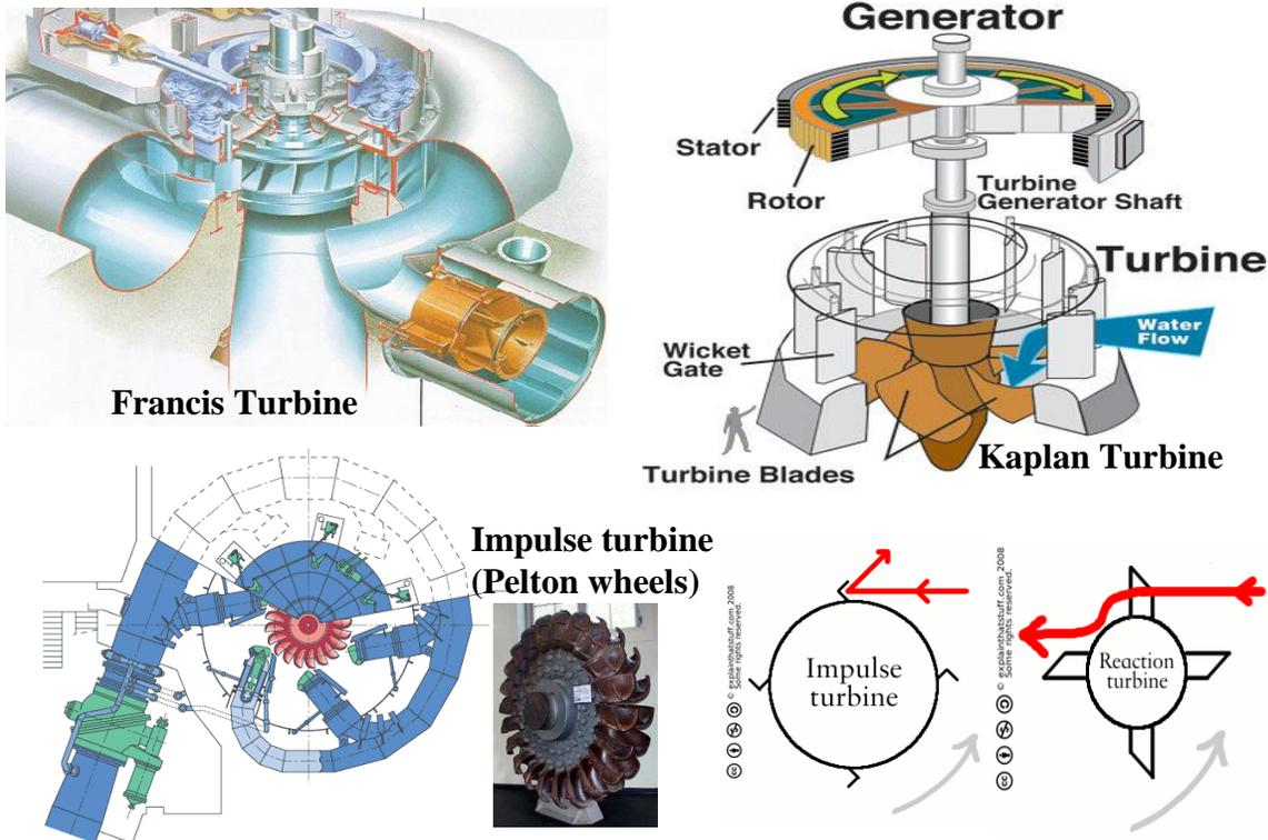
Fig. 12a: Reaction and impulse turbines
