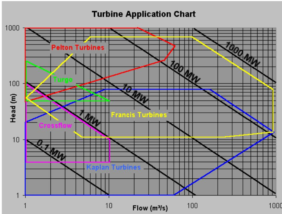
Fig. 12b: Typical application ranges of different hydro turbine types
