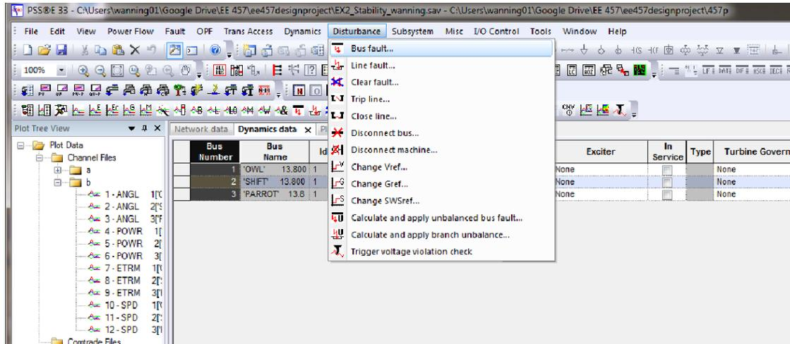
2) Then in the “Apply a But Fault” window, Click **Select** option and choose bus 103 and then press OK. See figure below
