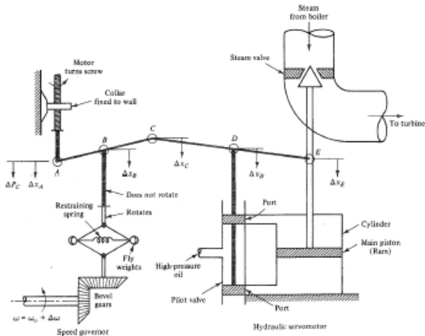
Figure 11.1 Servo-assisted speed governor.
