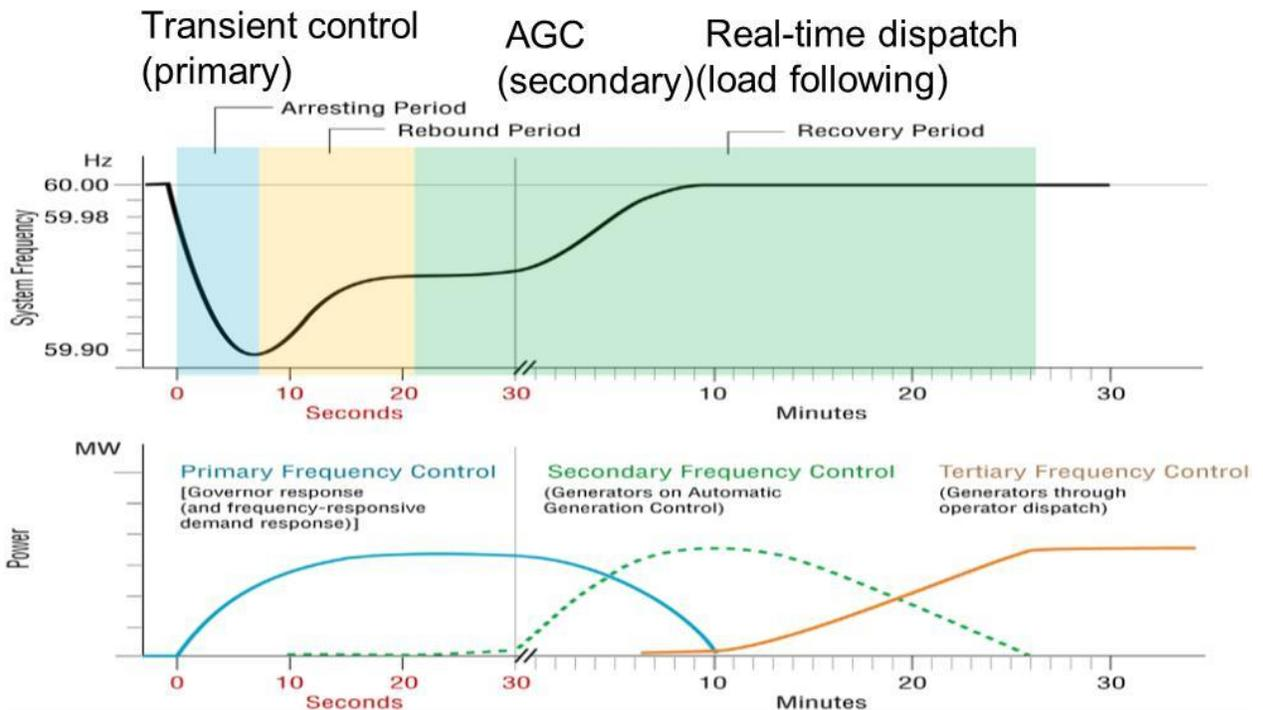
Fig. 2d: Transient & post-transient time frames
