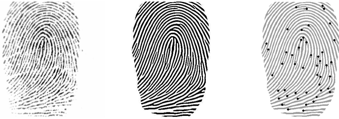
Figure 2: Feature Extraction Process: (a) original image, (b) after edge detection, (c) including feature points
