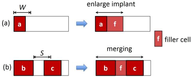
Fig. 2. Filler cell insertion to fix intra-row MinIA violations.
