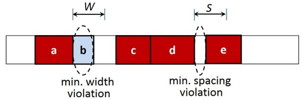
Fig. 1. Intra-row minimum implant width and spacing constraints.
