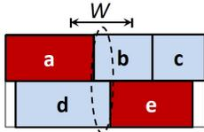
Fig. 4. Inter-row minimum implant width constraint.
