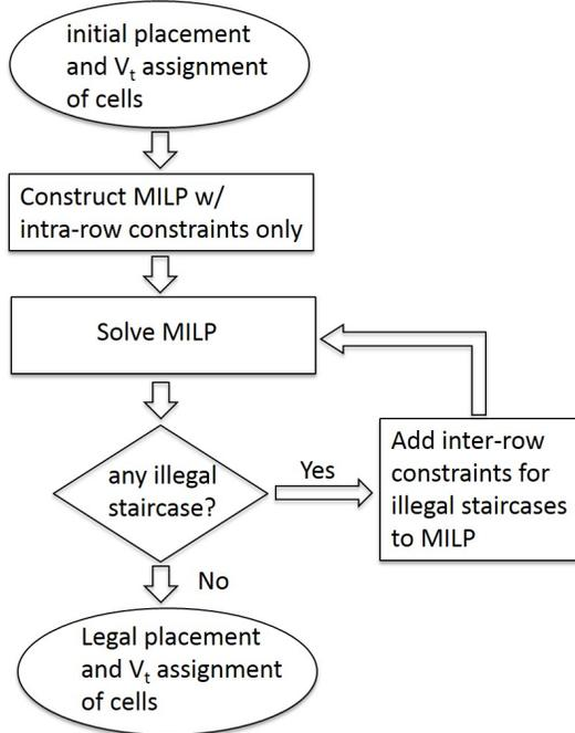
Fig. 7. The proposed technique to add inter-row constraints to our MILP on an as-needed basis.
