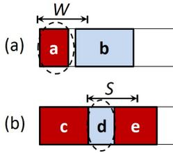
Fig. 3. Examples of intra-row MinIA violations that cannot be fixed by filler cell insertion.
