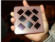
POWER5 chief scientist Balam Sinharoy holding a POWER5 MCM (Multi-chip Module)
