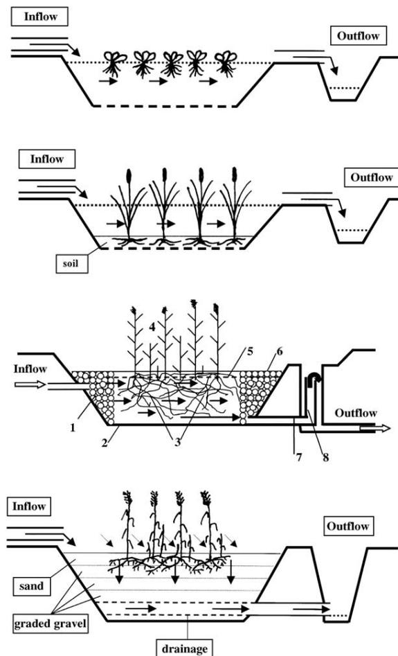
Figure 1 – The various types of constructed wetlands (Vymazal, 2006).
