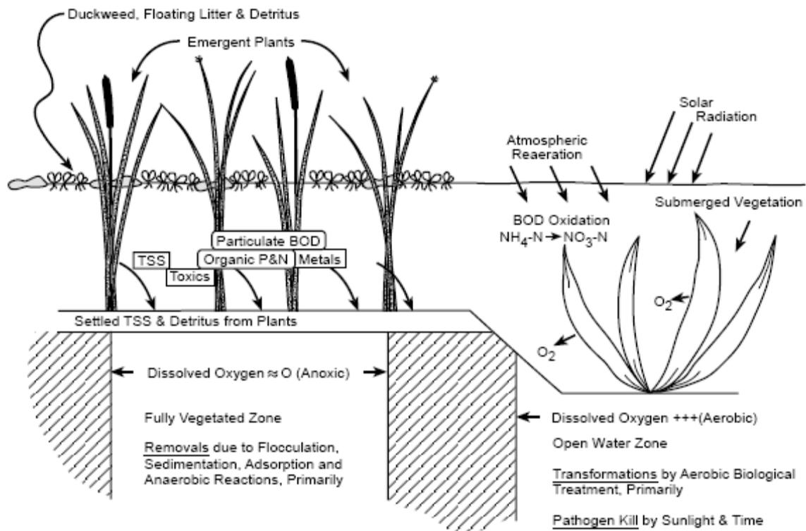
Figure 2 – Mechanisms present in a FWS wetland (EPA, 1999).
