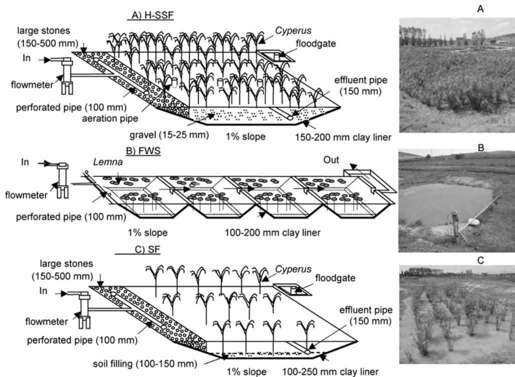
Figure 6 - The three different types of constructed wetlands used in the pilot study (Tuncsiper, 2007).
