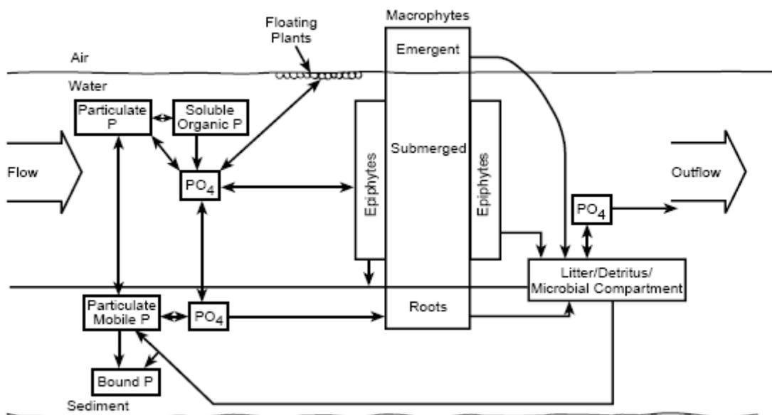
Figure 5 – Phosphorus transformations in a FWS wetland (EPA, 1999).
