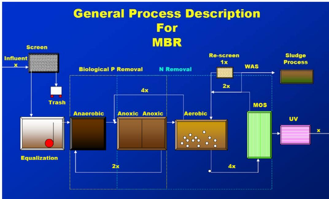
**Figure 4: MBR Biological Phosphorous Removal Design (www.usfilter.com)**
