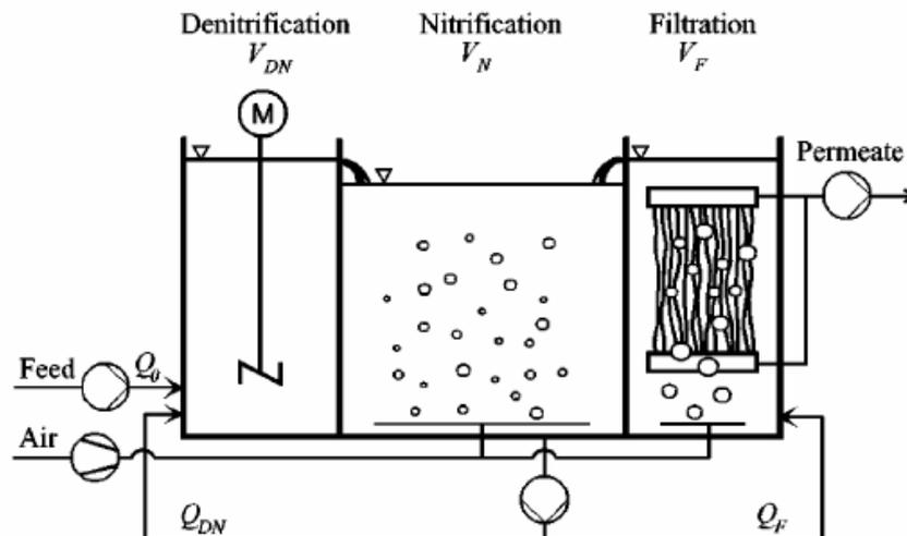
Figure 5: Pilot Municipal Treatment MBR Process Schematic (Rosenberger et al, 2002)
