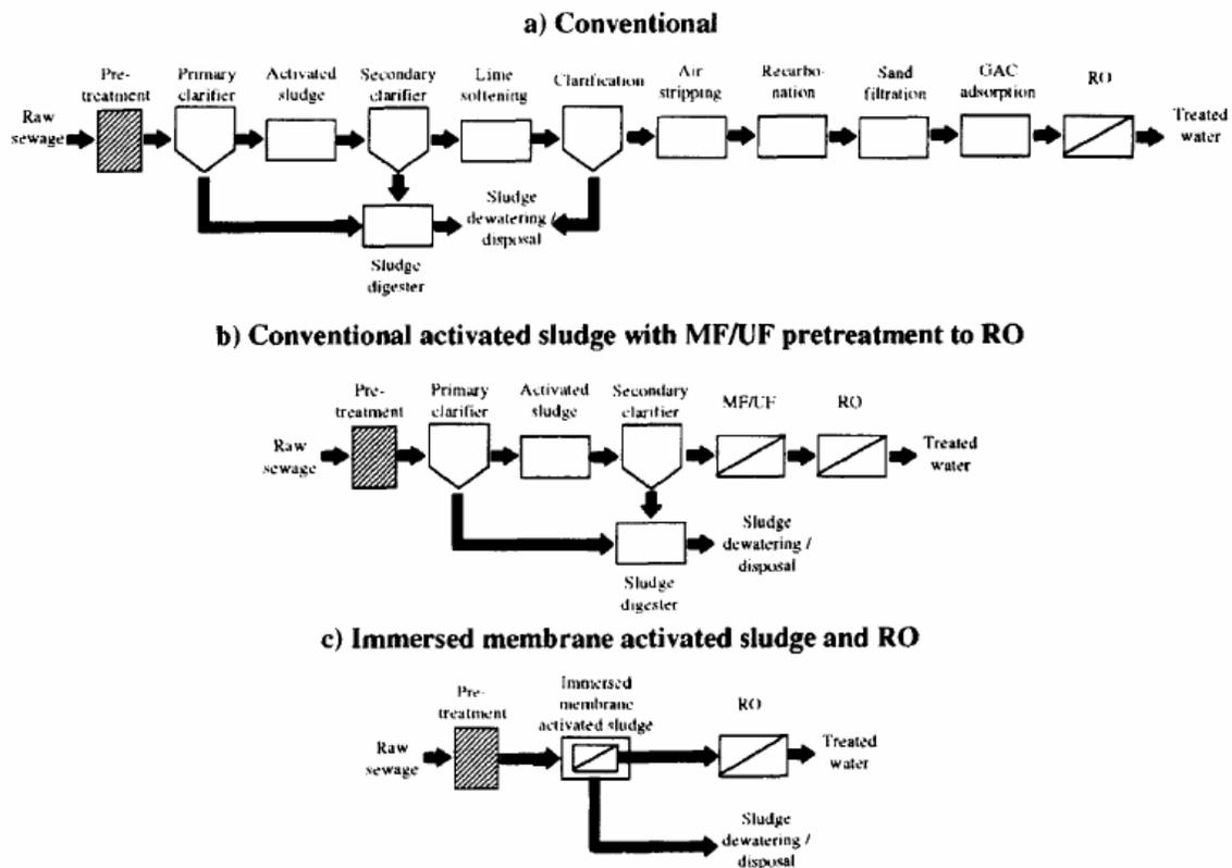
Figure 2: Comparison of Conventional and Membrane Treatment Trains (Cote, et al., 1997)
