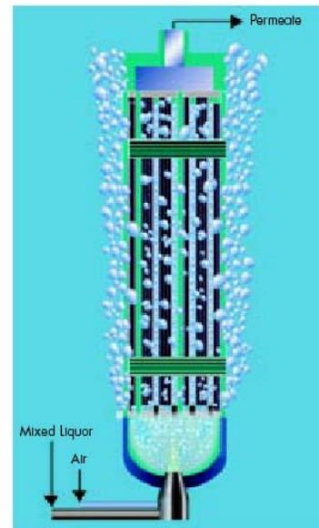
**Figure 11: USFilter Hollow Fiber Membrane Module Rack and Memjet System ([www.usfilter.com](http://www.usfilter.com))**
