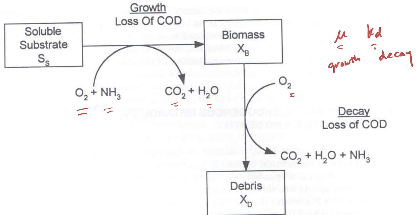
**Figure 3.5** Schematic representation of the traditional approach to modeling biomass decay and loss of viability.
