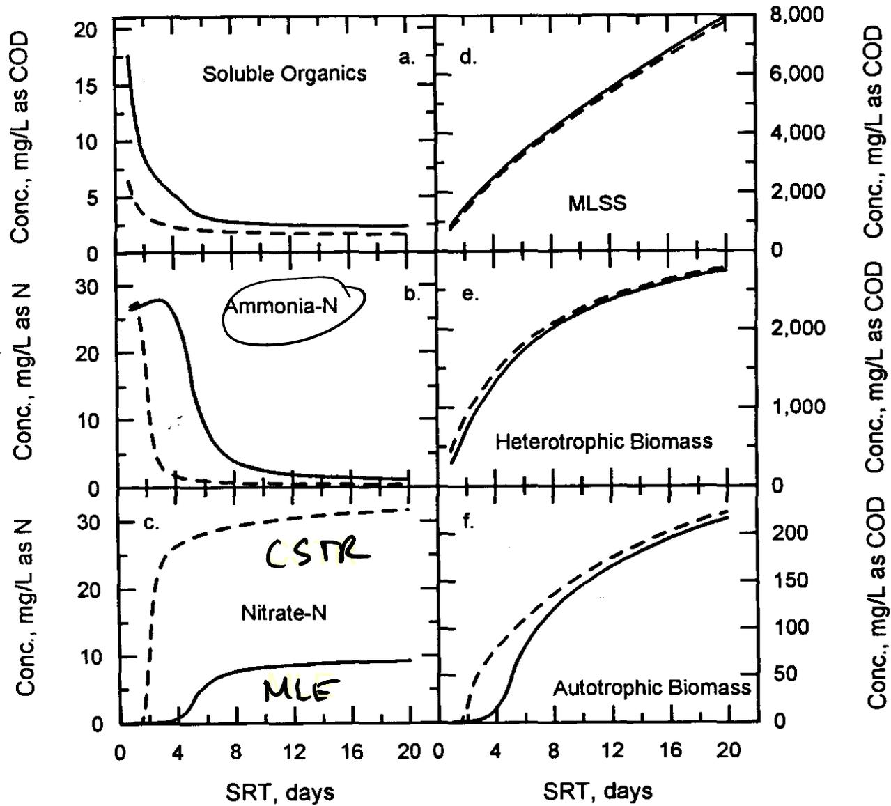
Dashed lines indicate performance of a single CSTR of the same volume as the anoxic and aerobic reactors.
