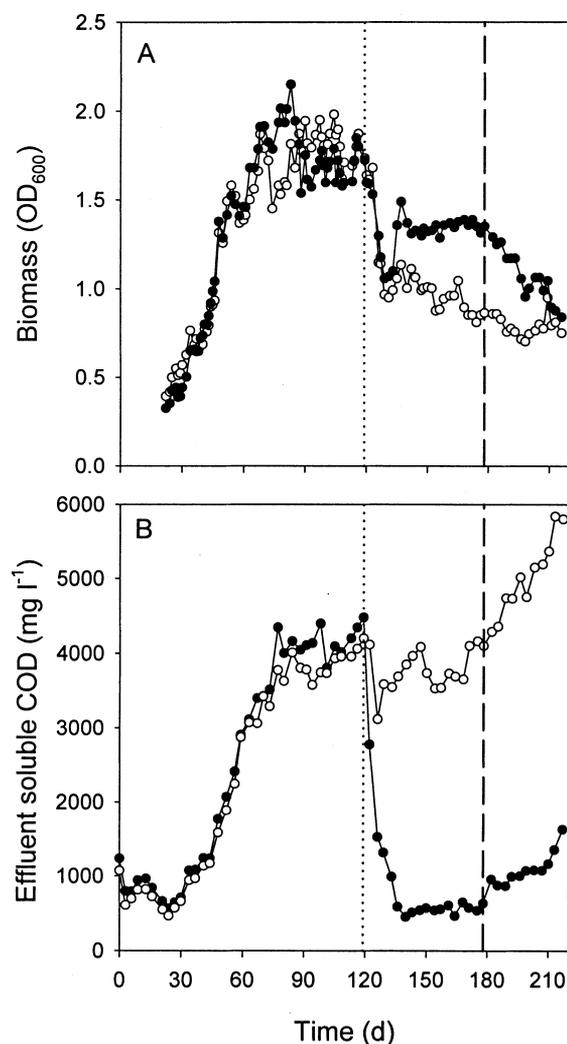
**Figure 1.** Biomass concentrations in the bulk fluid measured as optical density (A) and the effluent soluble COD concentrations (B) of a membrane-augmented anaerobic bioreactor (●) and a control anaerobic bioreactor (○) measured as optical density. The dotted and dashed lines indicate the dates when membrane aeration was initiated (day 119) and ammonium chloride was removed from the feed media (day 178), respectively.
