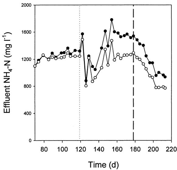
**Figure 2.** The effluent ammonium-nitrogen concentrations of a membrane-augmented anaerobic bioreactor (●) and a control anaerobic bioreactor (○). The dotted and dashed lines indicate the dates when membrane aeration was initiated (day 119) and ammonium chloride was removed from the feed media (day 178), respectively.
