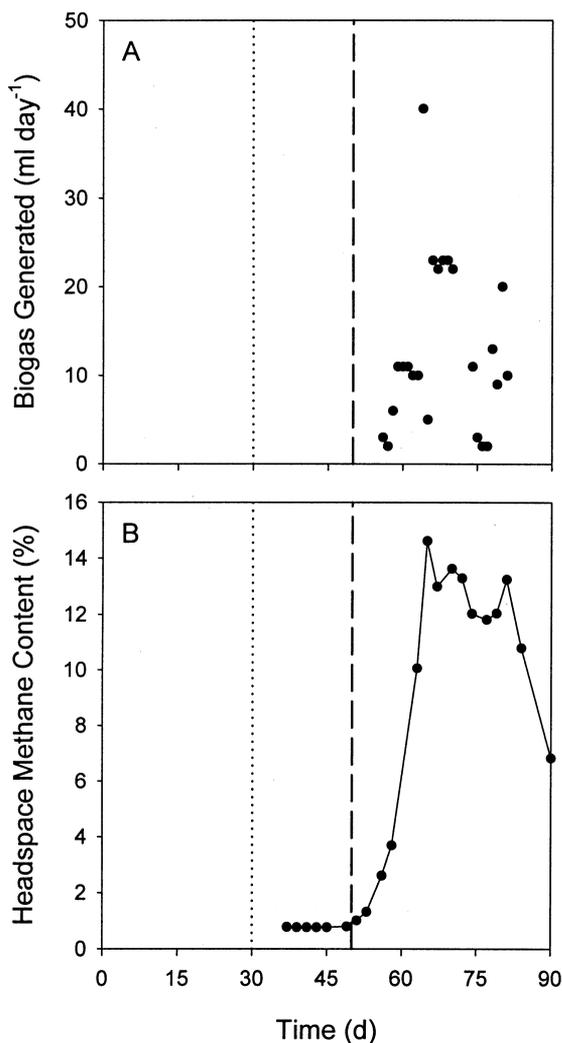
**Figure 8.** **A:** The quantity of biogas released from a membrane-augmented anaerobic bioreactor. **B:** The methane content of the headspace of a membrane-augmented anaerobic bioreactor.
