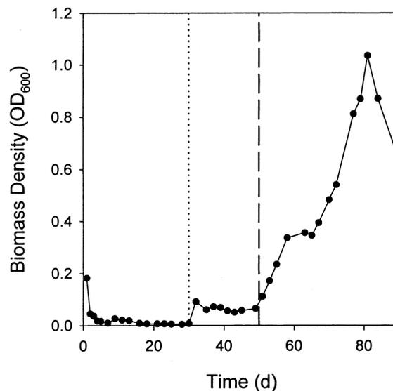
**Figure 7.** Biomass concentrations in the bulk fluid of a membrane-augmented anaerobic bioreactor measured as optical density. The dotted and dashed lines indicate the dates when the organic content of the feed medium was increased to 0.5 × strength (COD = 5,500 mg l<sup>-1</sup>) and 1.0 × strength (COD = 11,000 mg l<sup>-1</sup>), respectively.
