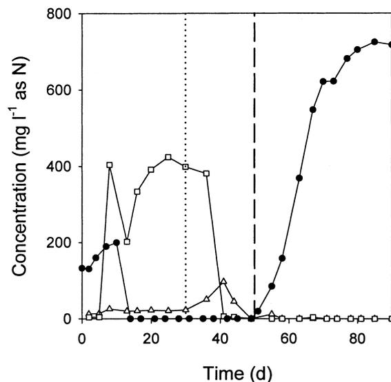
**Figure 6.** The concentrations of nitrogenous species in a membrane-augmented anaerobic bioreactor. The dotted and dashed lines indicate the dates when the organic content of the feed medium was increased to 0.5 × strength (COD = 5,500 mg l<sup>-1</sup>) and 1.0 × strength (COD = 11,000 mg l<sup>-1</sup>), respectively. ●, ammonium-nitrogen; □, nitrite-nitrogen; △, nitrate-nitrogen.
