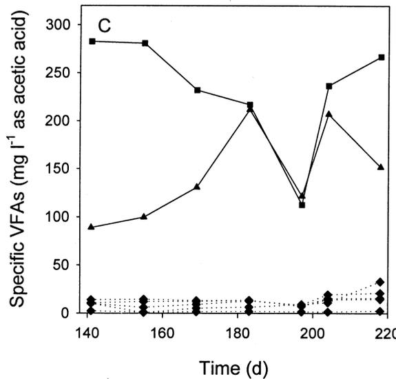
**Figure 4.** A: The total concentration of volatile fatty acids in the effluents from a membrane-augmented anaerobic bioreactor (●) and a control anaerobic bioreactor (○) following the initiation of membrane aeration. B: The concentrations of individual fatty acids in the effluent of a membrane-augmented anaerobic bioreactor. C: The concentrations of individual fatty acids in the effluent of a control anaerobic bioreactor. ■, acetic acid; ▲, butyric acid; ◆, all other organic acids.
