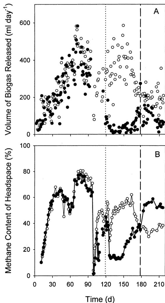
**Figure 5.** A: The quantity of biogas released from a membrane-augmented anaerobic bioreactor (●) and a control anaerobic bioreactor (○). B: The methane content of the headspace of a membrane-augmented anaerobic bioreactor (●) and of a control anaerobic bioreactor (○).
