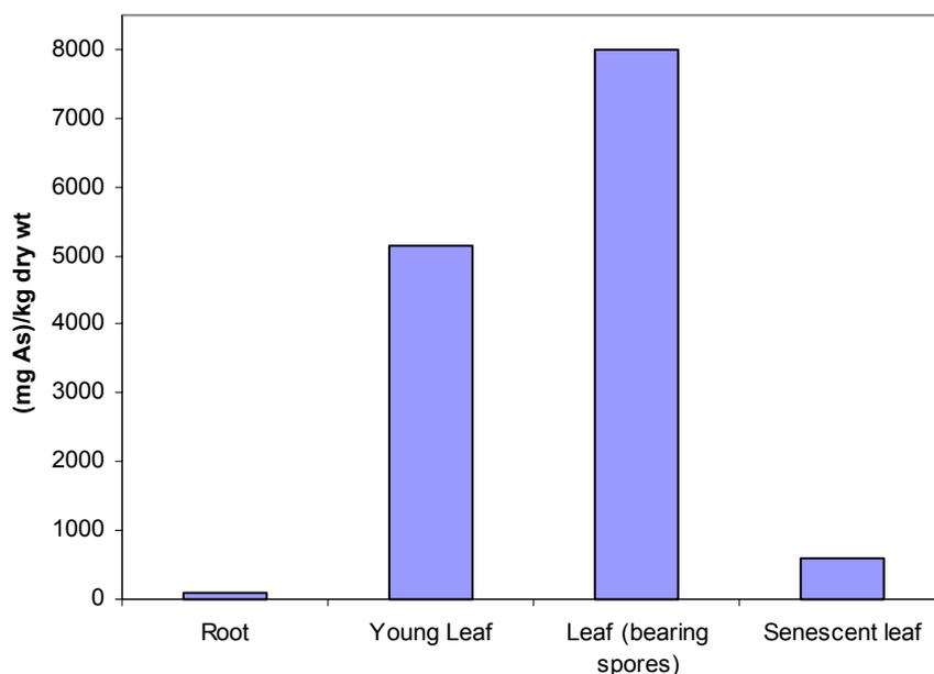
**Figure 2.** Concentration of arsenic per kg dry weight of *P. calomelanos* for different regions of the plant (Visoottiviset et al., 2002).
