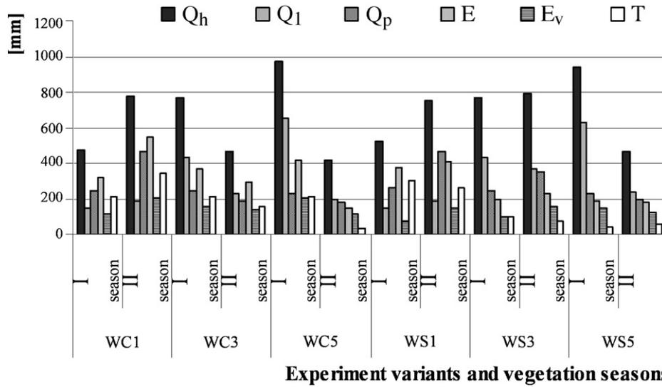
Fig. 2 – A comparison of the amount of water dozed into the lysimeters with the vaporization values. The description of the abbreviations is presented in Fig. 1.
