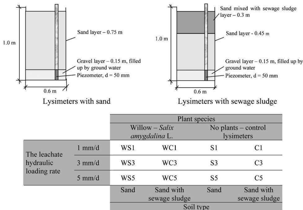
Fig. 1 – The construction of lysimeters and the experiment configuration.
