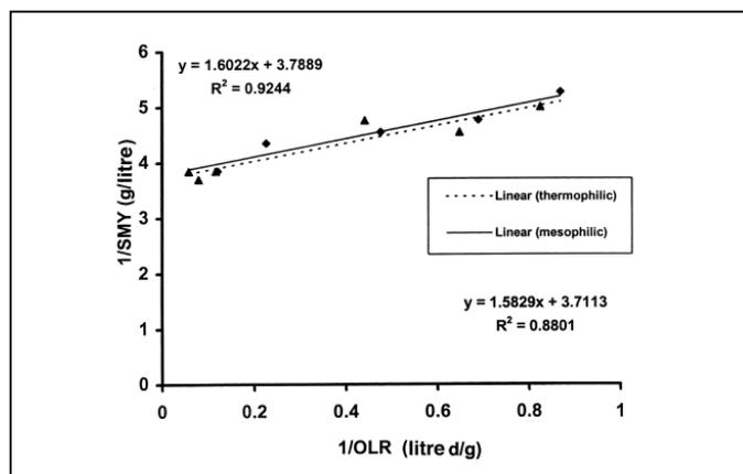
Figure 1. Determination of the Methane Production Kinetics: OLR is Organic Loading Rate in kg COD/m<sup>3</sup> day; SMY is Specific Methane Yield in m<sup>3</sup> CH<sub>4</sub>/kg COD Removed (Ahn and Forster, 2000)
