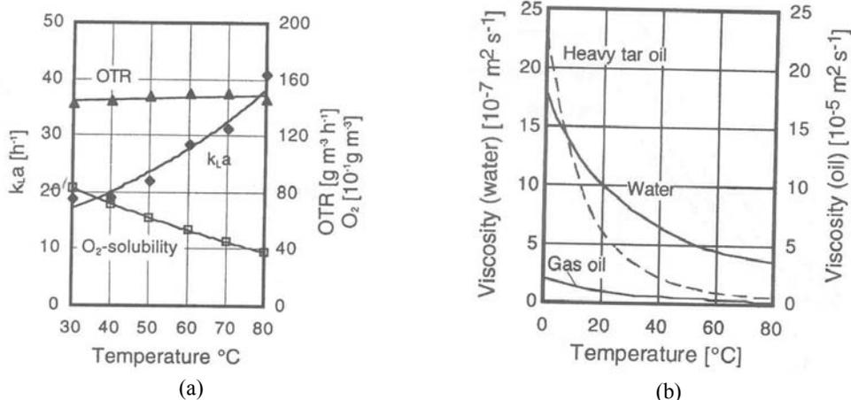
Figure 5 (a) Oxygen Transfer Efficiency (OTR), Oxygen Solubility and Overall Transfer efficiency ( $k_La$  at temperature T, °C (b) Viscosity of Water, Gas Oil and Tar Oil at varying temperature (Boogerd et al., 1990).
