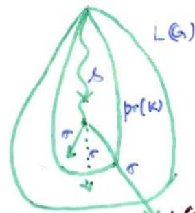
$s \in \text{pr}(K), \sigma \in \Sigma_u, s\sigma \in L(G) \Rightarrow s\sigma \in \text{pr}(K)$
