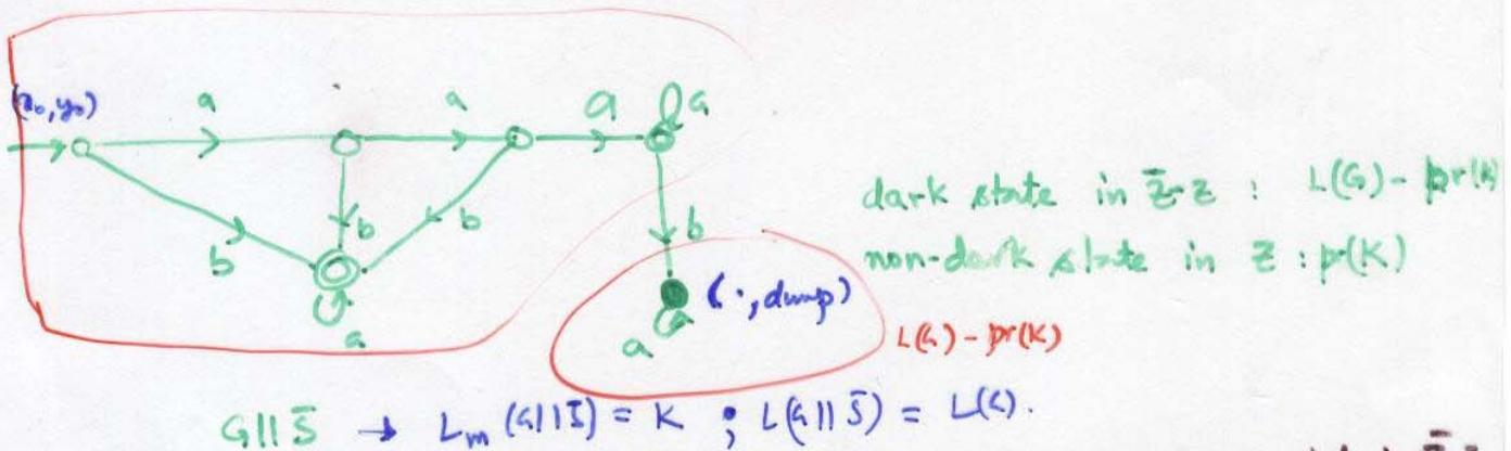
transition on uncontrollable event 'b' from a state in  $Z$  to a state in  $\bar{Z} - Z$
