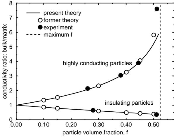
**Figure 3.** Bulk conductivity as a function of particle volume fraction for high-conductivity and insulating spherical particles in a low-conductivity matrix. The results of former theory are taken from [7] and the experimental data is taken from [16].
