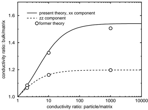
**Figure 7.** Bulk conductivity as a function of the particle/matrix conductivity ratio  $\alpha$  for oblate spheroids with aspect ratio 0.5,  $\alpha \geq 1$  and volume fraction 0.1. The results of former theory are taken from [7].
