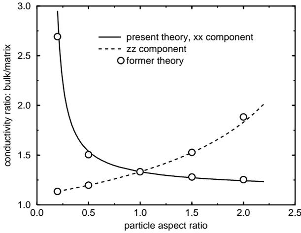
**Figure 6.** Bulk conductivity as a function of the particle aspect ratio  $\epsilon$  for high-conductivity particles and volume fraction 0.1. The results of former theory are taken from [7].
