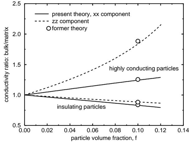
**Figure 4.** As for figure 3 but with prolate spheroidal particles with aspect ratio 2.0.
