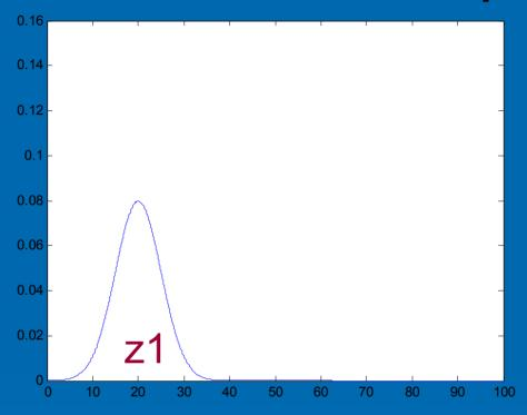
Sextant Measurement at t1: Mean = z1 and Variance =  $\sigma_{z1}^2$ Optimal estimate of position is:  $\hat{y}(t1) = z1$ Variance of error in estimate:  $\sigma_X^2(t1) = \sigma_{z1}^2$ Aircraft in same position at time t2 - <u>Predicted</u> position is z1
