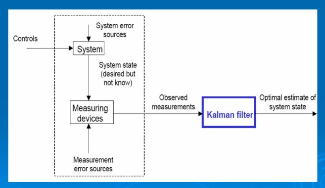
State cannot be measured directly. Has to be estimated Optimally from measurements
