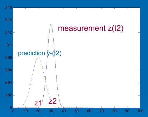
So we have the prediction  $\hat{y}$ -(t2) GPS Measurement at t2: Mean =  $z_2$  and Variance =  $\sigma_{z_2}^2$ Need to <u>correct</u> the prediction due to measurement to get  $\hat{y}$ (t2) Closer to more trusted measurement – linear interpolation?
