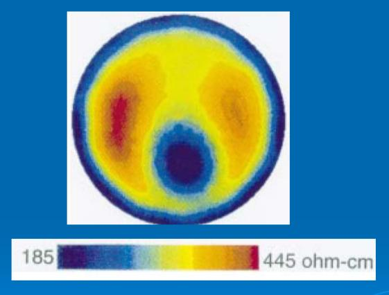
Impedance Map of the cross-section i.e. the resistivity distribution over the cross-section computed from measurements at the boundary Or the Circumference
