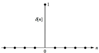
Figure 9: DT unit impulse. *Does not* correspond to sampled  $\delta(t)$ , CT unit impulse.
