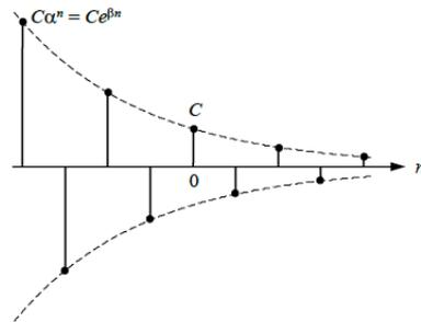
Figure 6: DT exponential functions for  $-1 < \alpha < 0$ .
