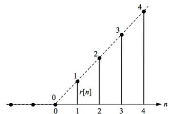
Figure 8: DT unit ramp. Corresponds to sampled  $r(t)$ , CT unit ramp.
