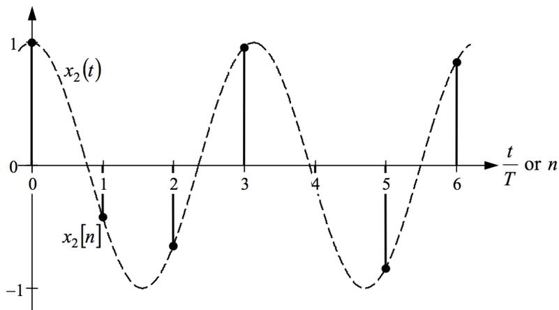
Figure 2:  $x_2(t)$  and  $x_2[n]$  in Example 2.*Frequency ambiguity*
