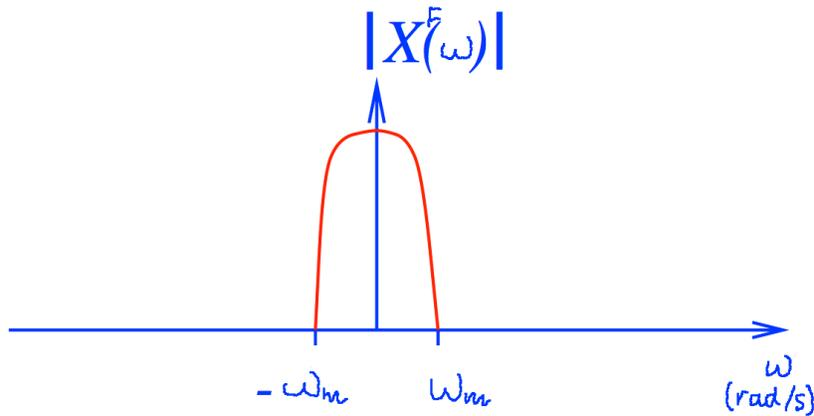
Figure 4: Spectrum of a lowpass CT signal  $x(t)$ .
