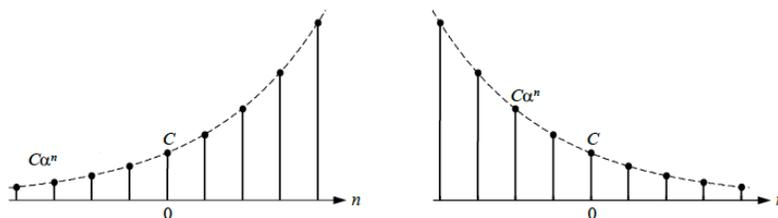
Figure 5: DT exponential functions for  $\alpha > 0$ .
