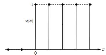
Figure 7: DT unit step. Corresponds to sampled  $u(t)$ , CT unit step.
