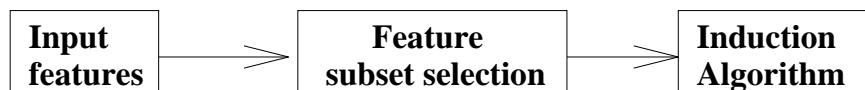
Figure 2: The feature filter approach, in which the features are filtered independently of the induction algorithm.
