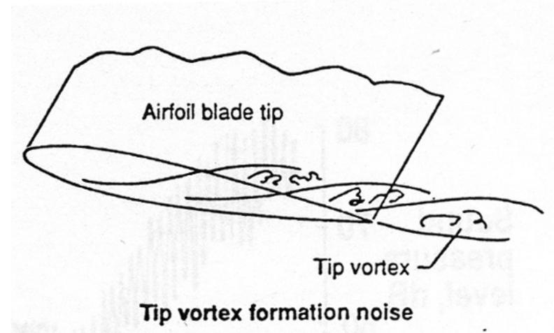
***$M^5$  noise scaling limits rotor size ... energy capture***
