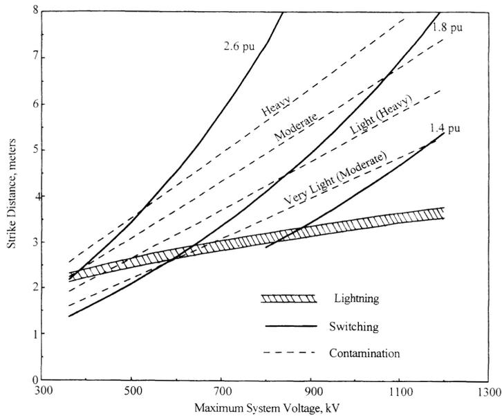
Figure 1.1:  $V_{50\%}$  Insulation Levels for Power Frequency Voltage, Switching Surges, and Lightning Surges
