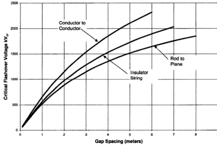
Figure 1.2:  $V_{50\%}$  Critical Flashover Voltages
