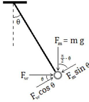
Figure 1.4: Blowout Pendulum Model
