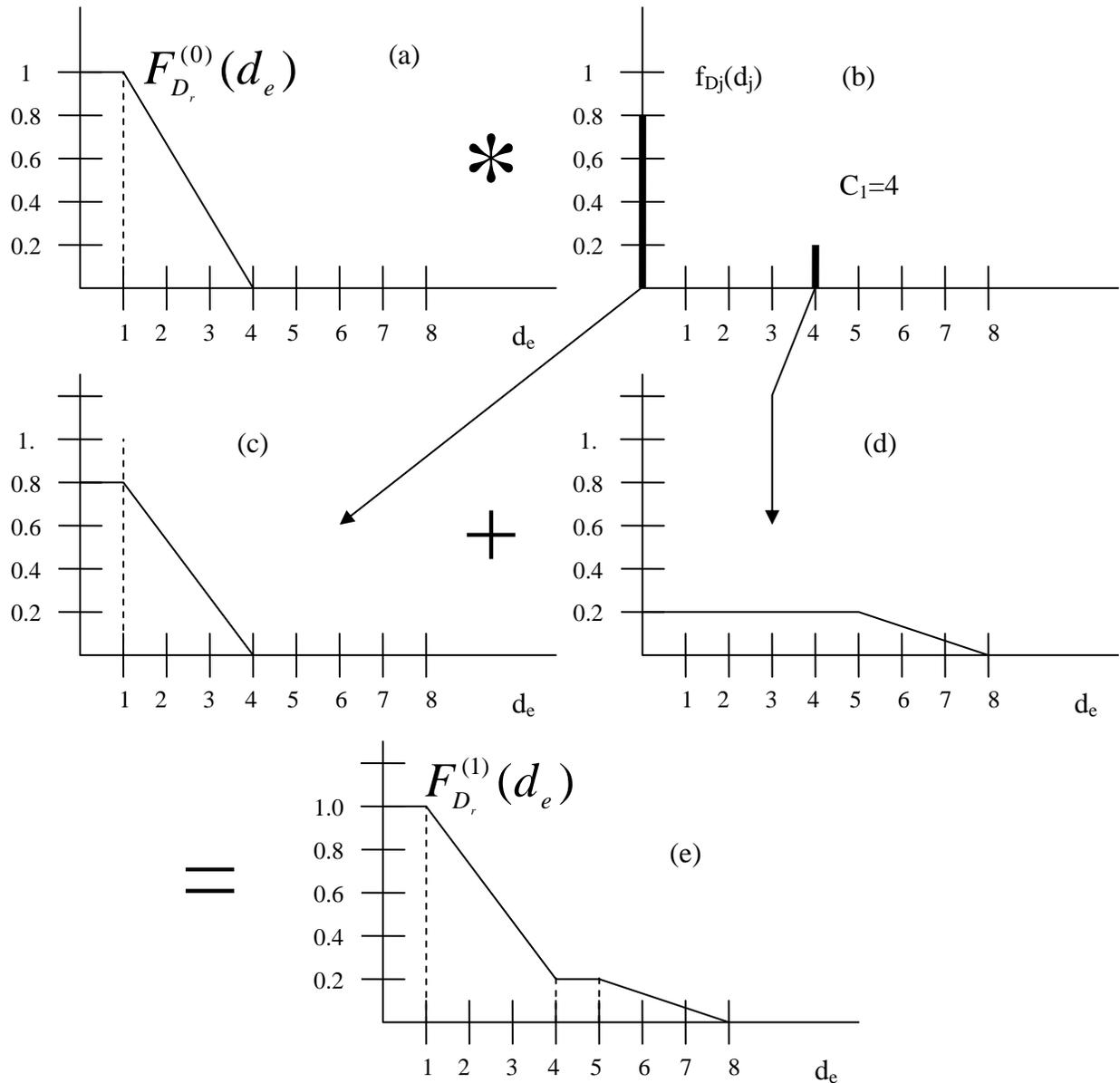
Fig. U19.21: Convolving in the first unit
