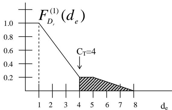
Fig. U19.23: Illustration of loss of load region
