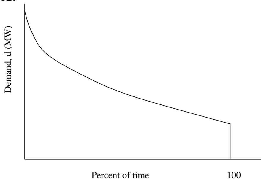
Fig. U19.12: Load duration curve
