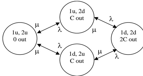
Fig. U19.6: State Space Model for 2-Unit System
