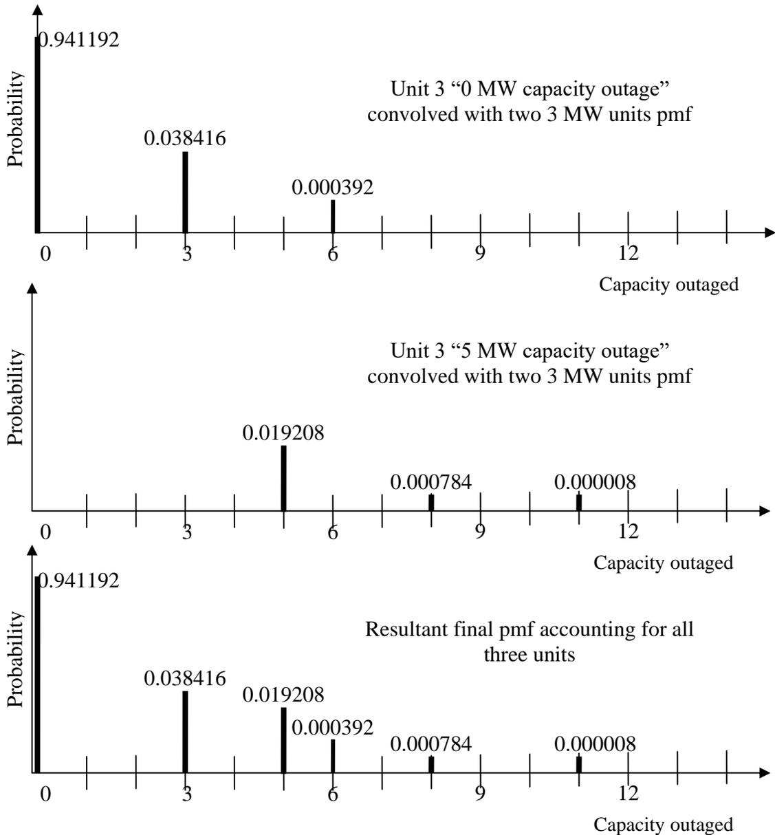
Fig. U19.10: Procedure for convolving Two 3 MW units with 5 MW Unit (top two plots) and final 3 unit pmf
