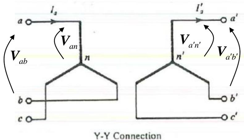
$$\frac{V_{an}}{V_{a'n'}} = \frac{\frac{1}{\sqrt{3}} V_{ab} \angle -30^\circ}{\frac{1}{\sqrt{3}} V_{a'b'} \angle -30^\circ} = \frac{V_{ab}}{V_{a'b'}}$$
