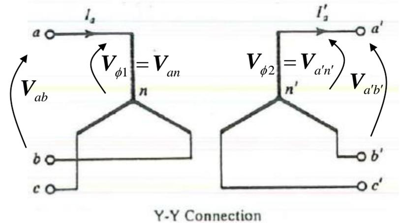
$$\frac{V_{ab}}{V_{a'b'}} = \frac{V_{\phi1}}{V_{\phi2}} = \frac{N_1}{N_2} \quad \text{This is ratio across phases}$$
