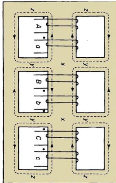
However, its mag circuit provides multiple paths for flux to flow; this reduces flux density seen by each leg which is advantageous for short-circuit performance (thermal & mechanical); so shell-types are used more frequently when high capacity is required.
