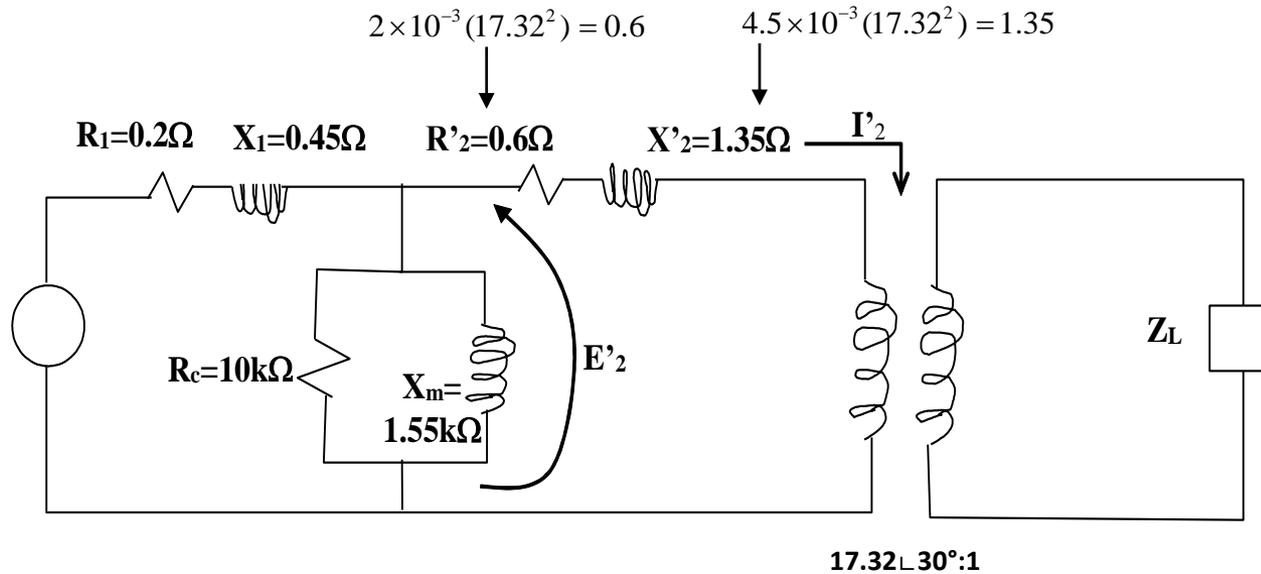
Observe here that for referring impedances we need only the magnitude of the effective turns ratio (and not phase). Reason for this is shown on Slide 12.
