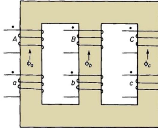
The shell-type requires more ferromagnetic material than does the core-type and so is typically more costly on a per-MVA basis.
