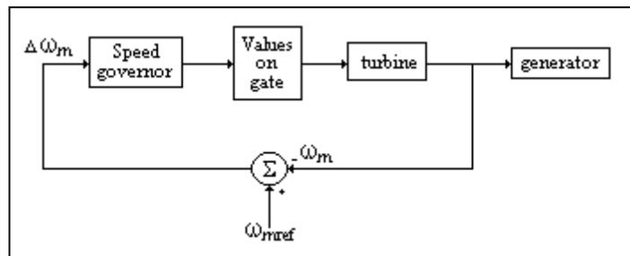
Figure G1.13 Block Diagram of Speed Governing Control System
