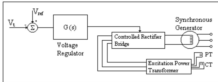
Figure G1.12 Static Type Excitation System
