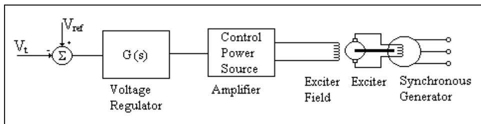
Figure G1.10 Rotating DC Commutator Type Excitation System
