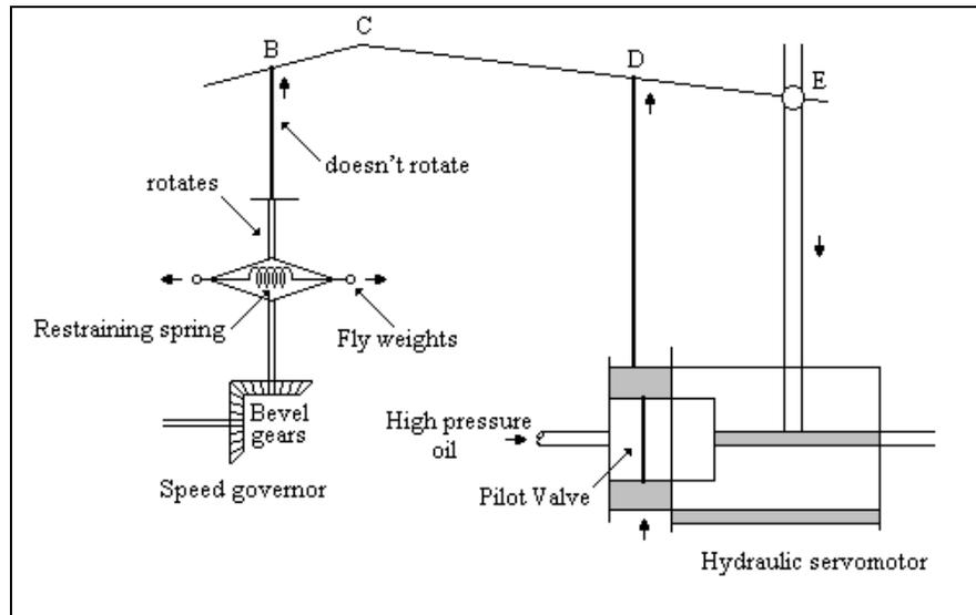
Figure G1.14 Mechanical-Hydraulic Governor Design
