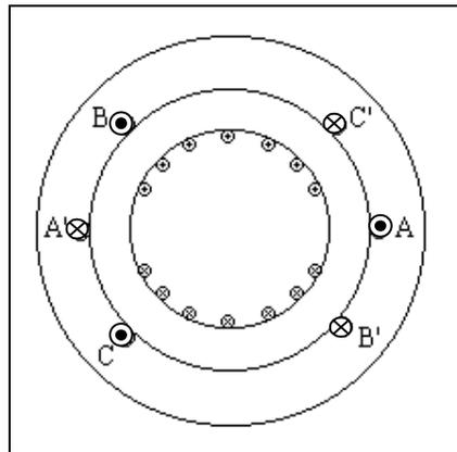
Figure G1.3 Winding Layout for Two-Pole Smooth Rotor Synchronous Machine
