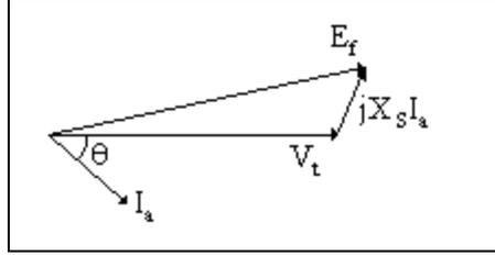
Figure G1.6 Phasor Diagram for Equivalent Circuit – Inductive Load
