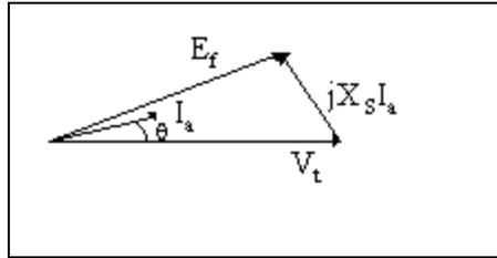
Figure G1.7 Phasor Diagram for Equivalent Circuit – Capacitive Load
