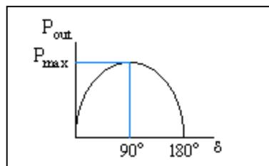
Figure G1.8 Power Angle Curve
