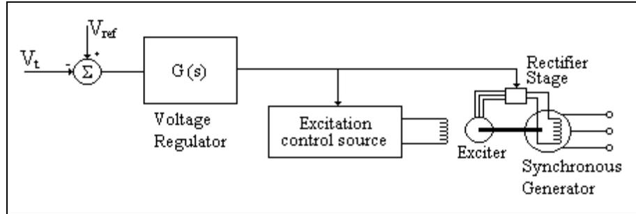
Figure G1.11 Rotating AC Alternator Type Excitation System
