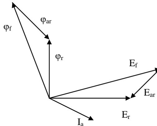
Figure G1.4 Phasor Diagram for Synchronous Machine
