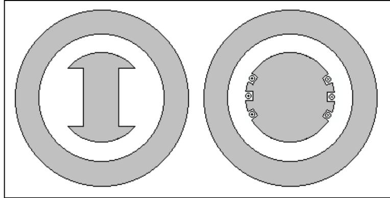
Figure G1.2 Salient Pole (left) and Smooth (right) Rotor Construction
