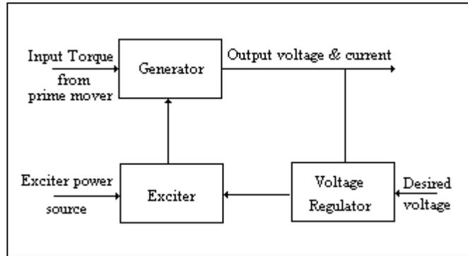
Figure G1.9 Block Diagram of Excitation Control System
