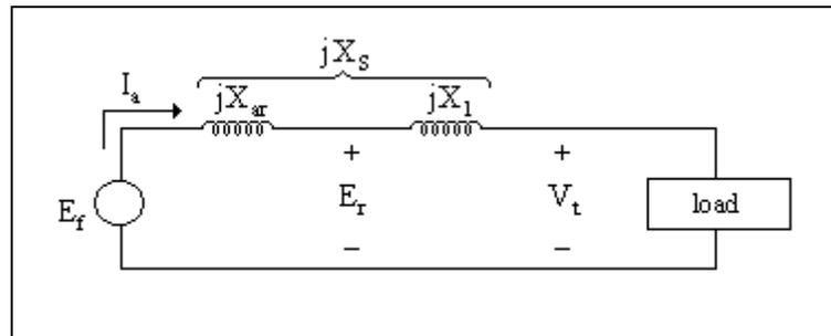
Figure G1.5 Equivalent Circuit Model of Synchronous Machine
