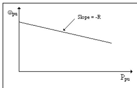
Figure G1.15 Steady-State Droop Characteristic
