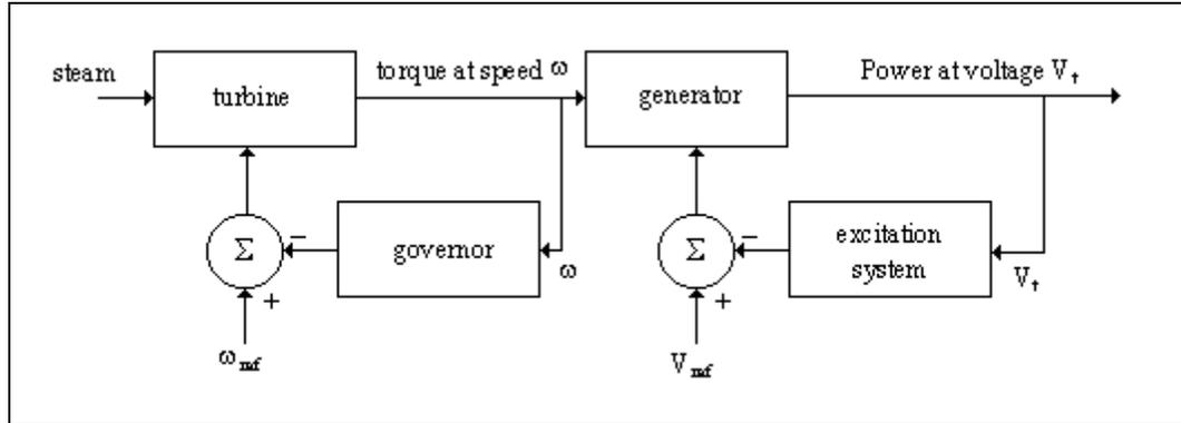
Figure G1.1 Block Diagram for Turbine-Generator System
