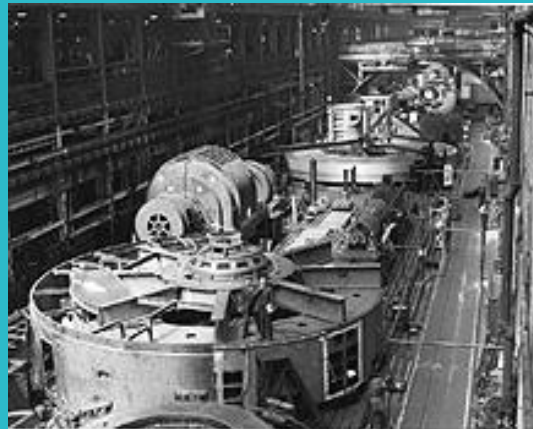
45,000 Kilovolt-ampere waterwheel for Tennessee Valley Authority (foreground), c.1938
