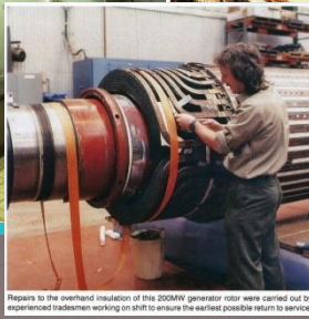
Repairs to the overhead insulation of this 200MW generator rotor were carried out by experienced tradesmen working on scaffolding to ensure the earliest possible return to service.
