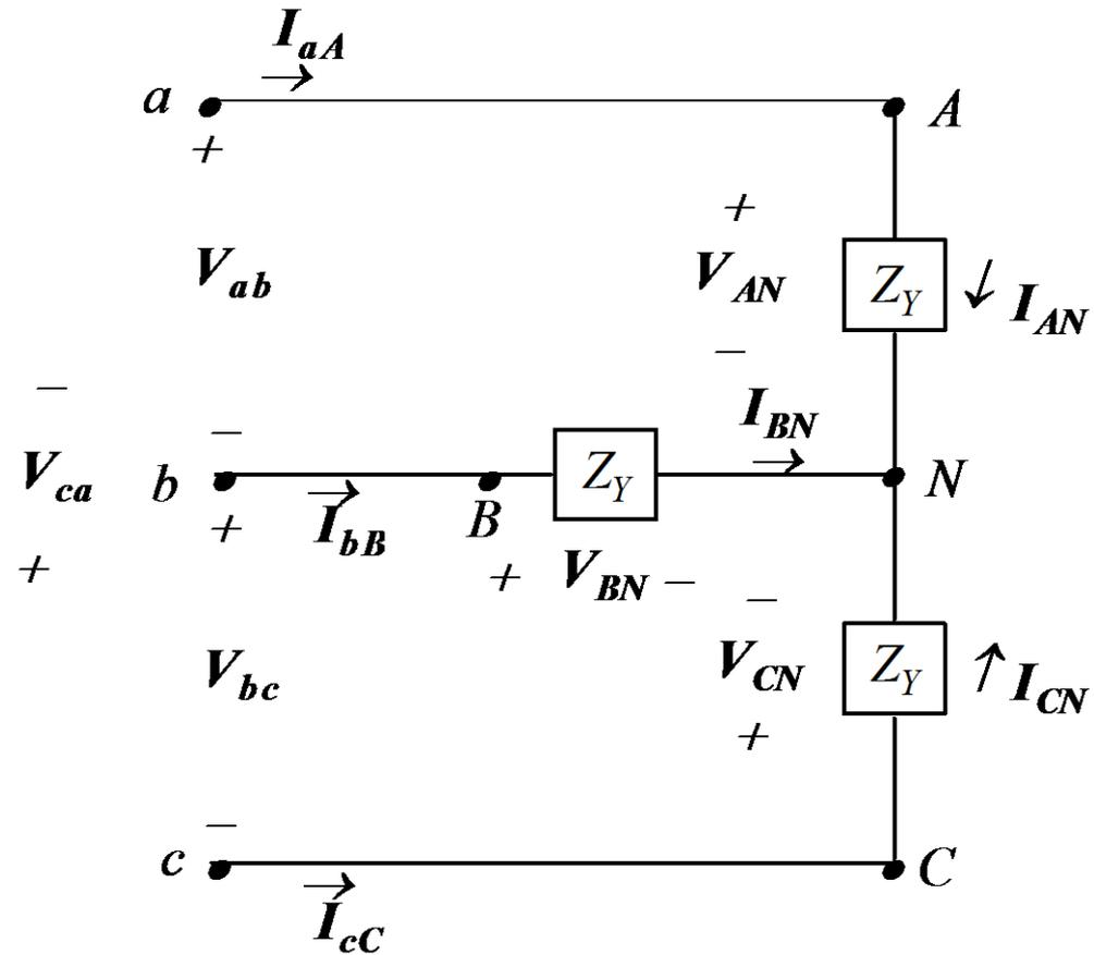
$I_{aA}$  is equal to the phase current  $I_{AN} = I_{\phi}$
