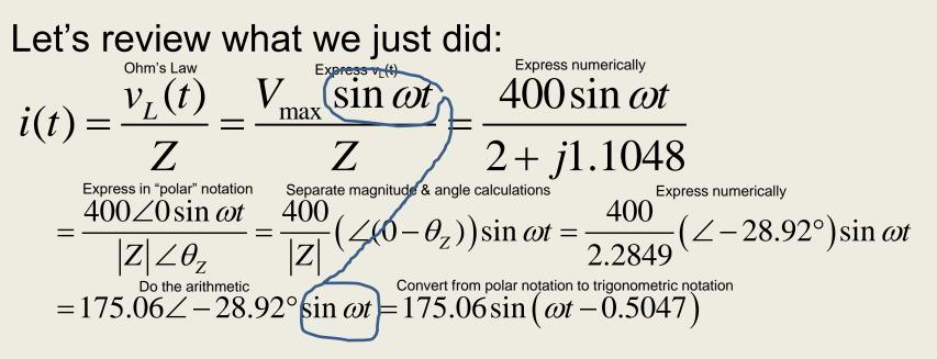
Notice that nothing ever happened to the  $\omega$ t part. Nor did the sinusoidal function change. This means that the frequency of the current is the same as the frequency of the voltage. If this is the case, then why do we need to carry the sin $\omega$ t through the calculations? Why not just drop it? This is what we do when we use <u>phasor notation</u>, as in the next slide.
