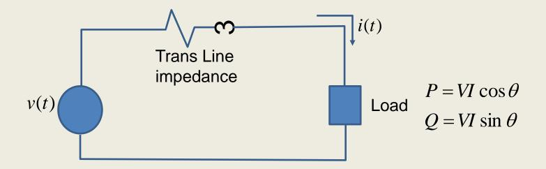
Assume V is constant, and we must supply P (this is the real power of the load). With V and P constant, from P=VIcos $\theta$ , Icos $\theta$ =I×pf must be constant. What do we want pf to be?
