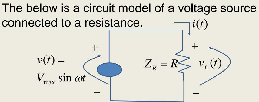
We apply Kirchoff's Voltage Law (KVL): the sum of voltages around the loop must be 0:  $v(t) - v_L(t) = 0$  $\Rightarrow v_L(t) = v(t)$
