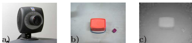
Figure 3.5 The robot’s vision system: a) a closeup of the 3D camera; b) a color image of a red non-container captured by the camera when mounted on the robot; c) the depth image corresponding to b).
