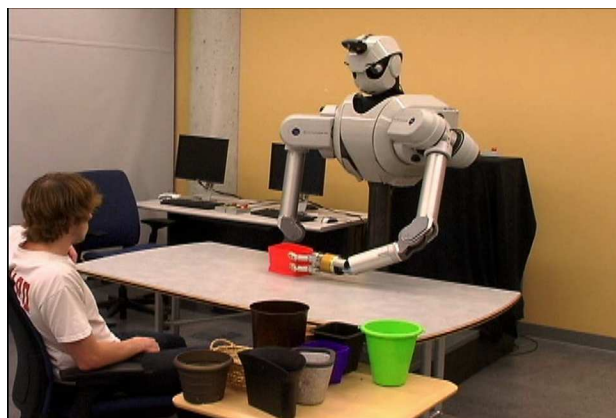
Figure 3.1 The upper-torso humanoid robot used in this thesis, shown here moving a container. Objects were placed on the table before each trial by the experimenter.
