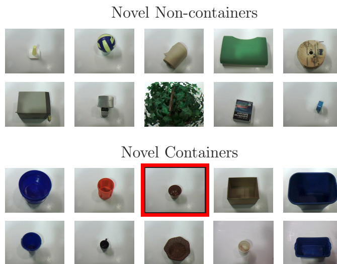
Figure 4.7 The result of using a Nearest Neighbor classifier to label novel objects as ‘containers’ or ‘non-containers’. The flower pot (outlined in red) was the only misclassified object. Sparse coding features were extracted from the 10 training objects and used in the classification procedure.
