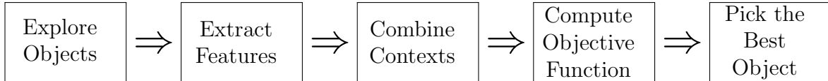
Figure 1.1: The framework used by the robot to solve perceptual reasoning tasks that involve multiple objects. The steps are as follows: 1) The robot explores the objects; 2) It extracts features from the raw sensory data it collected; 3) The robot combines the information from each of the sensorimotor contexts; 4) It computes the value of a task-specific objective function for each candidate solution; and 5) The robot selects the candidate that maximizes the objective function.
