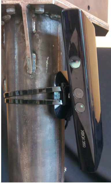
Figure 3.5: The robot’s Microsoft Kinect RGBD camera. It was attached to the metal stand supporting the robot during the experiments described in Chapter 6.
