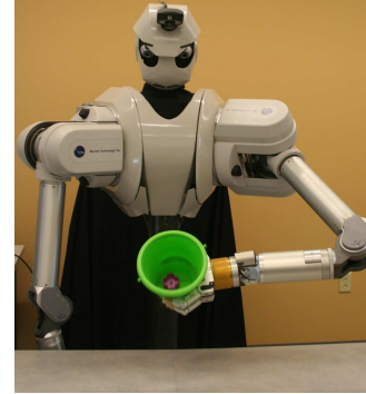
Fig. 1. The upper-torso humanoid robot used in the experiments. The robot is shaking one of the container objects used in the experiments.
