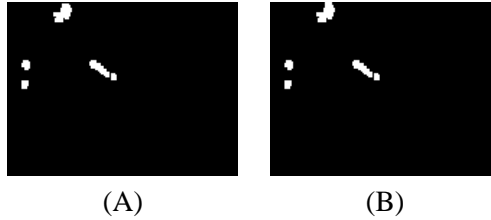
Figure 2: Using conditional dilation to combine two measurements. The resulting images show location of the head and the two hands. (A) Color and motion energy combined. (B) Color and stereo depth map combined. These are very similar in this instance. This similarity vanishes when the camera and subject both move as shown by later examples.
