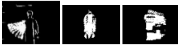
Figure 4: 3 examples of motion energy profiles used for training NN used for gesture recognition.
