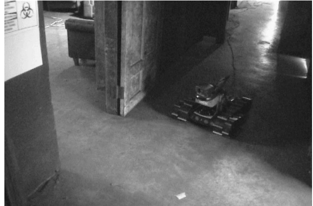
Figure 8: The RWI Urban Robot equipped with a SICK laser scanner and a Sony pan/tilt/zoom camera.
