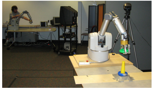
Figure 4: Remote arm being controlled by the user in the top left corner. During experiments, a screen prevented the user from seeing the remote arm. The camera on the right provided visual feedback.
