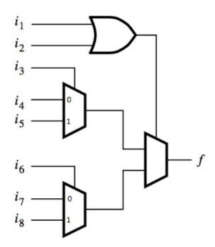
**P7** (10 points). Implement this function using only 4-to-1 multiplexers and no other logic gates
